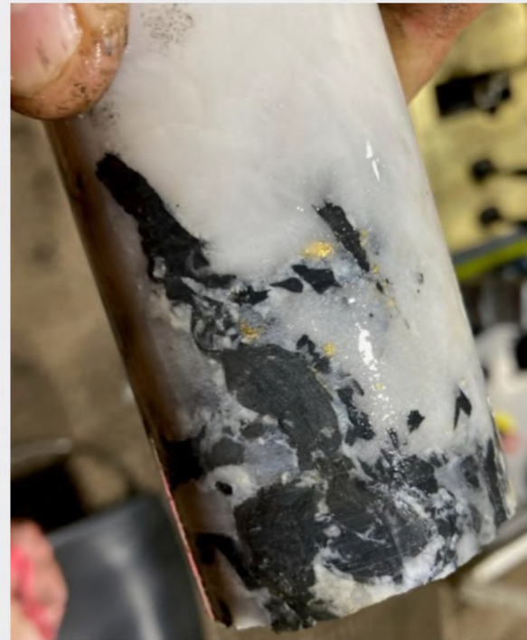
BMDD001W1 – visible gold at 544.9m in intercept 1.2m @ 543g/t Au from 544.2m
