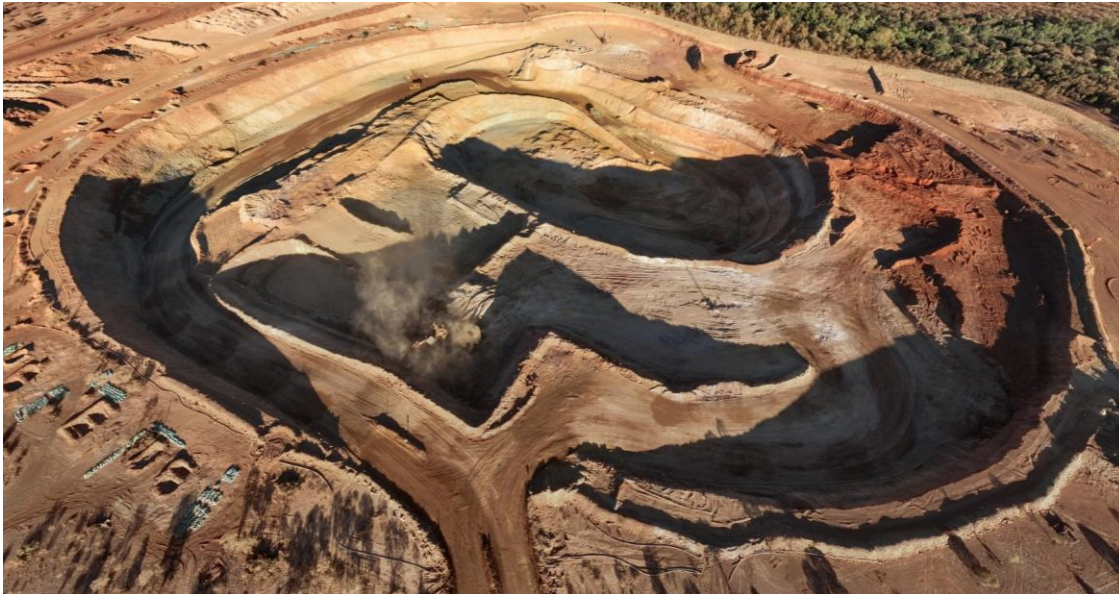
Progression of CP Stage 1 pit inside larger Stage 2 pit boundary 31 January 2026
