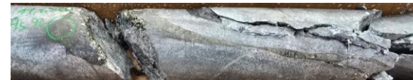
Chalcopyrite sulphide within a c-type vein within altered porphyry from 400m in 25LHDD0070
