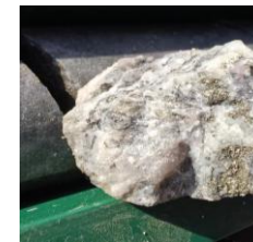
Pyrite-Chalcopyrite-Molybdenite sulphide veining from 1,351m downhole in 25LHDD071
