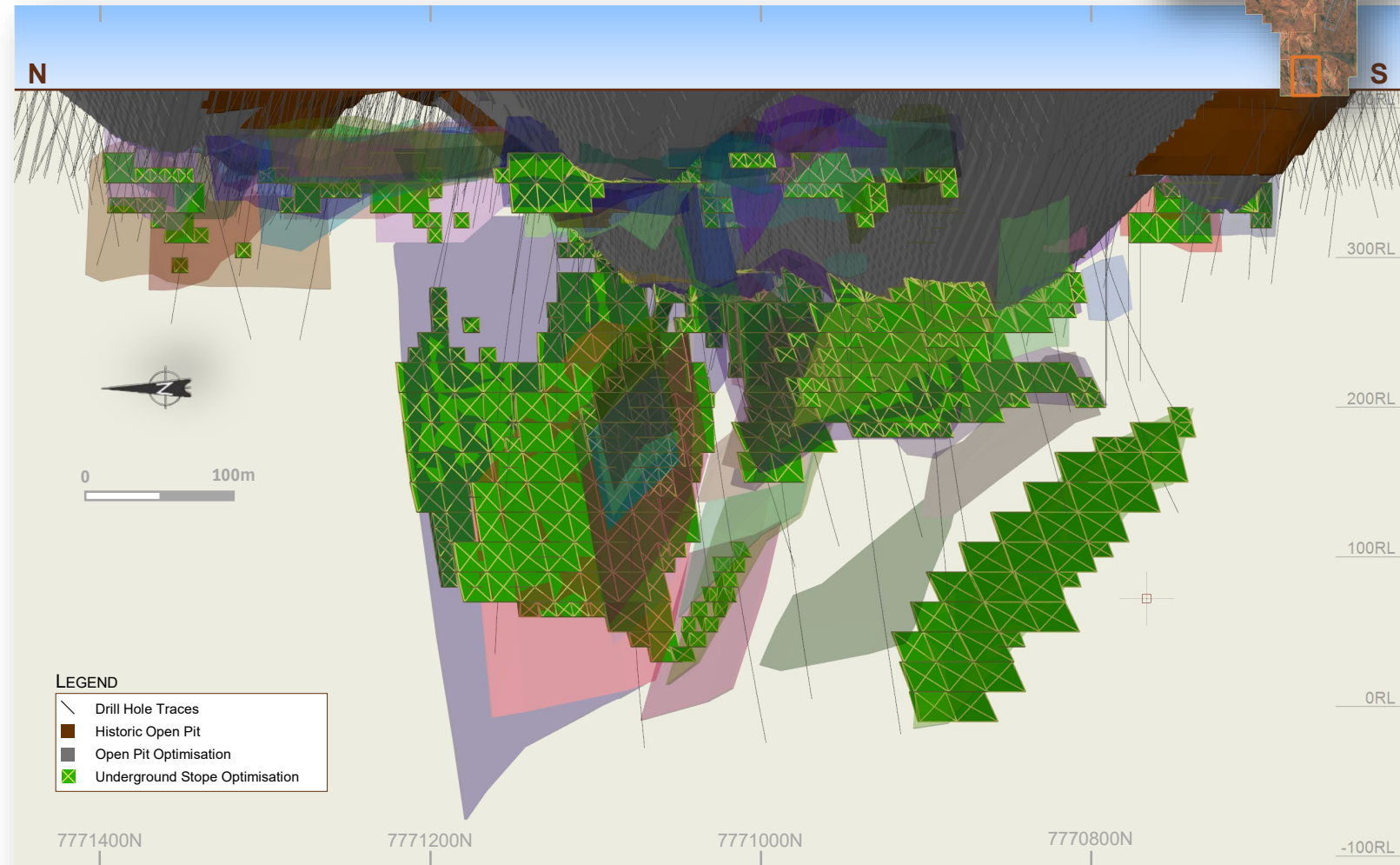
Above: Long section looking East-South-East, showing the Existing Pit (Brown), pit shell (grey), stope optimisation (green) and MRE wireframes
