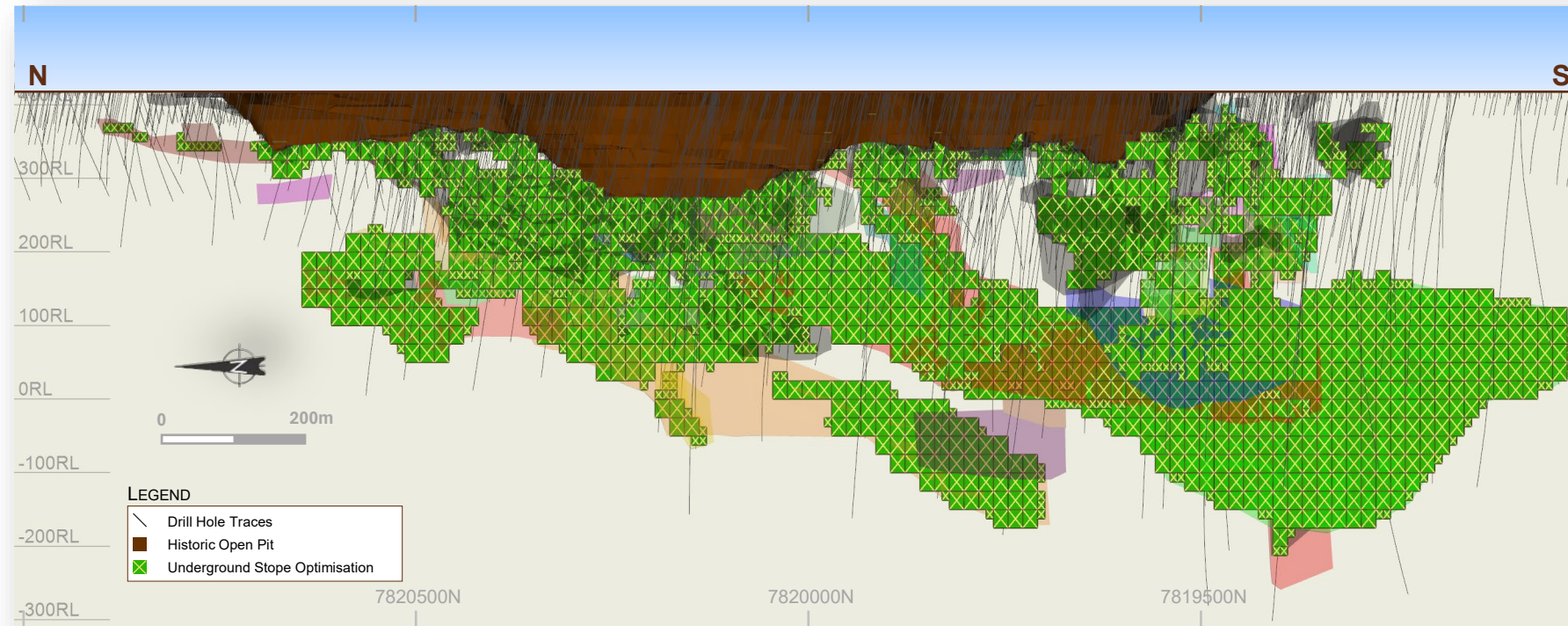
Above: Long section looking East-North-East, showing the Existing Pit (Brown), pit shell (N/A), stope optimisation (green) and MRE wireframes
