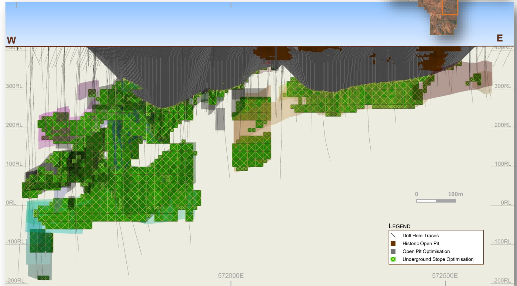
Above: Long section looking North-North-West, showing the Existing Pit (Brown), pit shell (grey), stope optimisation (green) and MRE wireframes
