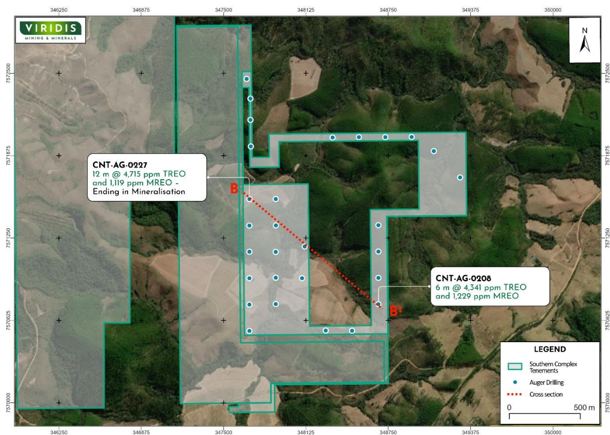
Figure 4: Southern Complex (South Area) – plan view of auger drilling on a 200 m x 200 m reconnaissance grid within the greenfield area acquired by Viridis in the most recent ANM tenement auction, showing selected significant intercepts (TREO and MREO).
