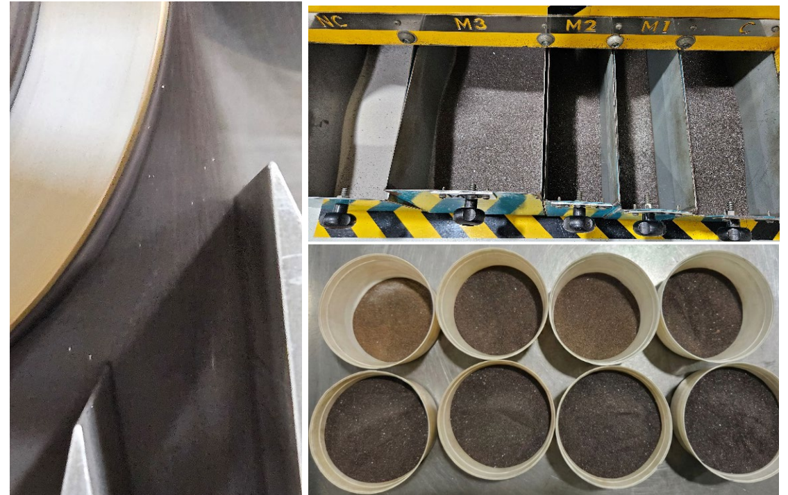
Rosewood RM01 material undergoing magnetic and electrostatic separation. Left - roll magnetic separation, Top Right - products from one of the electrostatic stages. Bottom Right – rare earth roll magnet separations.
