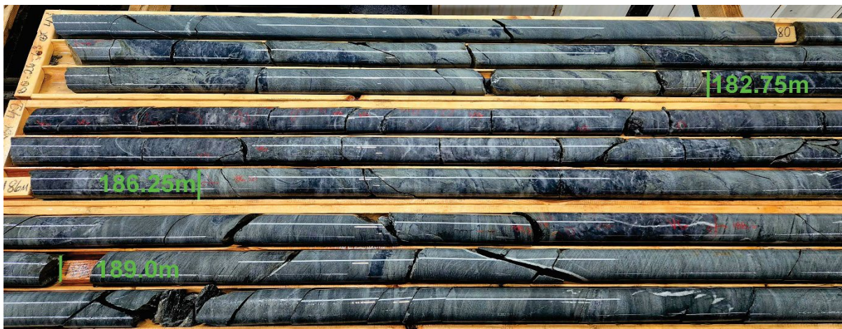
Figure 2 Core trays for BO-26-63 showing intercept of visual gold occurrences across the 6.25m interval from 182.75m. (Core Diameter 4.76cm, See Table 2 for detailed logs)
