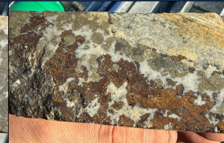
538.5 to 540.5m – 0.6g/t Au, 0.3% Cu, 1.1% Pb, 7.9% Zn and 13.6g/t Ag (6.0g/t AuEq 2 ).
