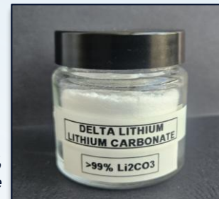
Mt Ida Lithium Carbonate 99.8% produced from mica concentrate
