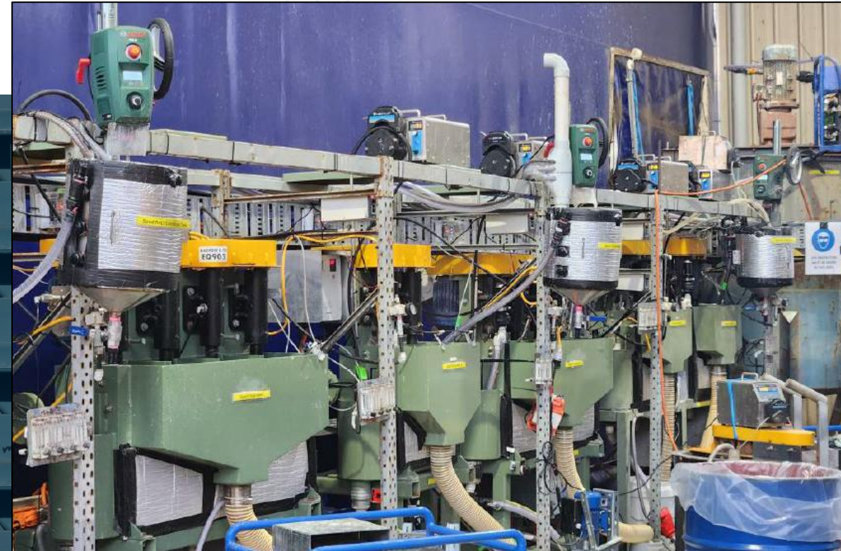
Pilot plant spodumene flotation circuit during operation
