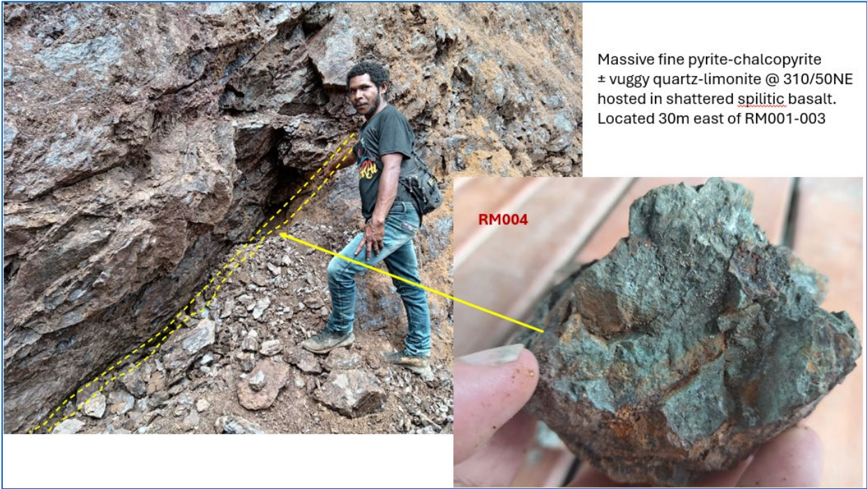
Photo 2: Massive pyrite-chalcopyrite vein in shattered “spilitic” basalt
