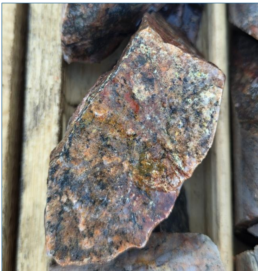
Figure 1: Photo of split core from drillhole PCDD25-014 (470462E, 5558025N, UTM Zone 21, sample ID H091491) demonstrating visual uraninite mineralisation along joint surfaces and along fractures in split drill core from at downhole depth of 28m. Laboratory analysis of a 1m interval including this sample returned 124 ppm U_3O_8 (refer to Appendix 1).
