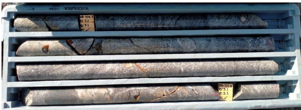
Figure 4: Photos of core from RRPT0002 showing multiple silica-sulphide (chalcopyrite and pyrite up to 1%) veins 104.6-107.9m, noting the oxidation of sulphides.
