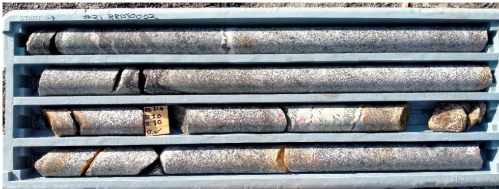
Figure 3: Photos of core from RRPT0002 showing multiple silica-carbonate-sulphide (chalcopyrite and pyrite up to 1% with 40% banded pyrite from 70.9m for 0.1m) veins 69.9-73.5m, noting the oxidation of sulphides.
