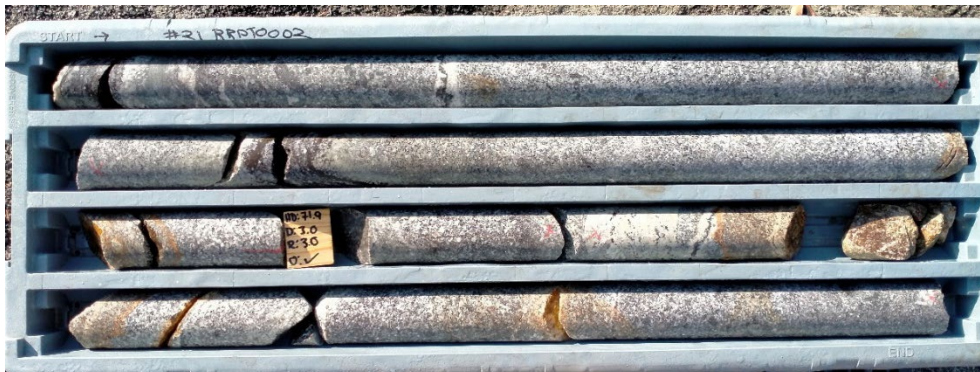
Figure 3: Photos of core from RRPT0002 showing multiple silica-carbonate-sulphide (chalcopyrite + pyrite) veins 69.9-73.5m, noting the oxidation of sulphides.
