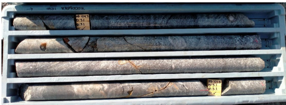
Figure 4: Photos of core from RRPT0002 showing multiple silica-sulphide (chalcopyrite + pyrite) veins 104.6-107.9m, noting the oxidation of sulphides.
