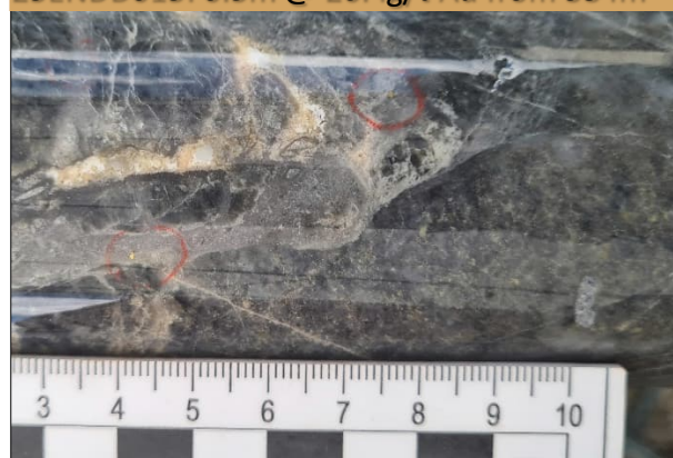
Photo 4. Visible gold (circled red) in hole 25ENDD015 at 384.47m down hole, which returned 0.5m @ 26.4g/t Au from 384m , in a quartz-iron carbonate-pyrite vein within strongly phyllic altered granite host rock. Scale bar units are centimetres.
