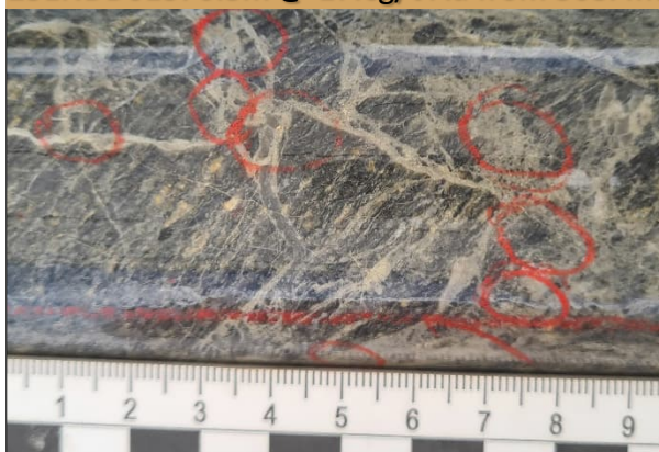
Photo 3. Visible gold (circled red) in hole 25ENDD015 at 368.55m down hole, which returned 0.3m @ 17.6g/t Au from 368.4m , in pyrite-quartz ± sulphosalts-arsenian pyrite-iron carbonate veins within moderately phyllic altered granite host rock. Scale bar units are centimetres.
