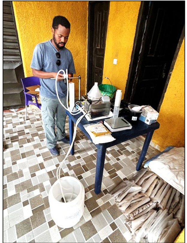
Figure 5. Photographs of SEMS PortablePPB field lab set-up in Zuénoula for rapid gold assaying of MGA soil samples
