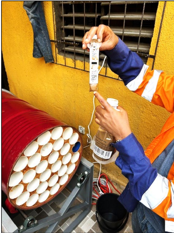
Figure 5. Photographs of SEMS PortablePPB field lab set-up in Zuénoula for rapid gold assaying of MGA soil samples
