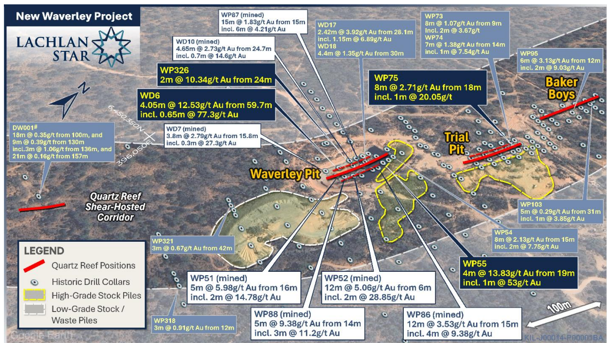
Figure 3: Oblique view (looking north-west) of the Waverley and Trial pits within Mining Lease M63/673, highlighting approximate position of gold-rich quartz reefs, significant intercepts and stockpiles/dumps.
