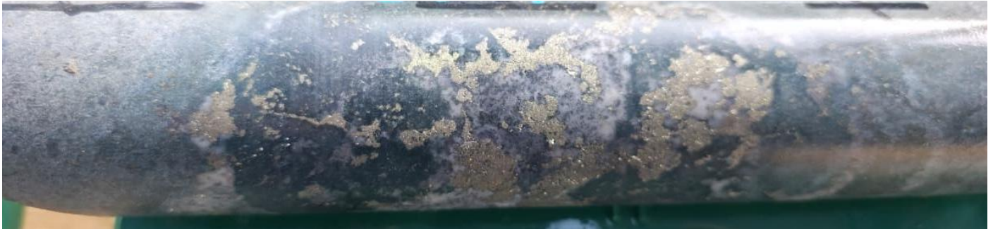
Photo 5. Pyrite-Chalcopyrite disseminated sulphide from 1,432m downhole in 25LHDD071* (refer to Appendix 1).
