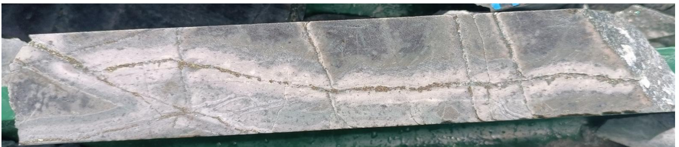
Photo 1. Pyrite-Chalcopyrite sulphide veining with albite selvage's from 1,434m downhole in 25LHDD071* (refer to Appendix 1).
