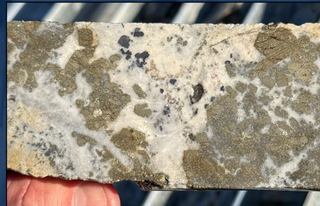
540.5 to 542.5m – 1.9g/t Au, 0.3% Cu, 1.1% Pb, 0.8% Zn and 17.3g/t Ag (3.6g/t AuEq 2 ).
