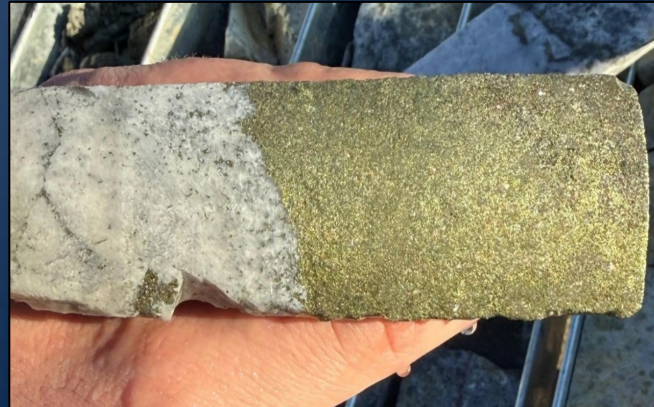
524.5 to 526.5m – 0.4g/t Au, 1.4% Cu, 0.2% Pb, 0.1% Zn and 15.5g/t Ag (3.3g/t AuEq 2 ).
