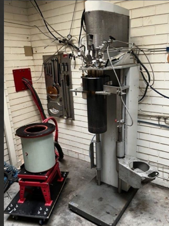
High-pressure autoclave with induction heater and control system being utilised for TP7
