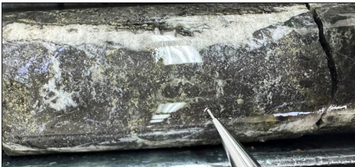
Figure 4. Core photograph from 383.8m to 386.2m in ZRSD25236, showing massive sulphides of sphalerite-galena-pyrrhotite-pyrite- chalcopyrite – 4.4 g/t Au, 0.3% Cu, 3.0% Pb, 3.5% Zn, 88.3 g/t Ag (9.2 g/t AuEq 2 ).
