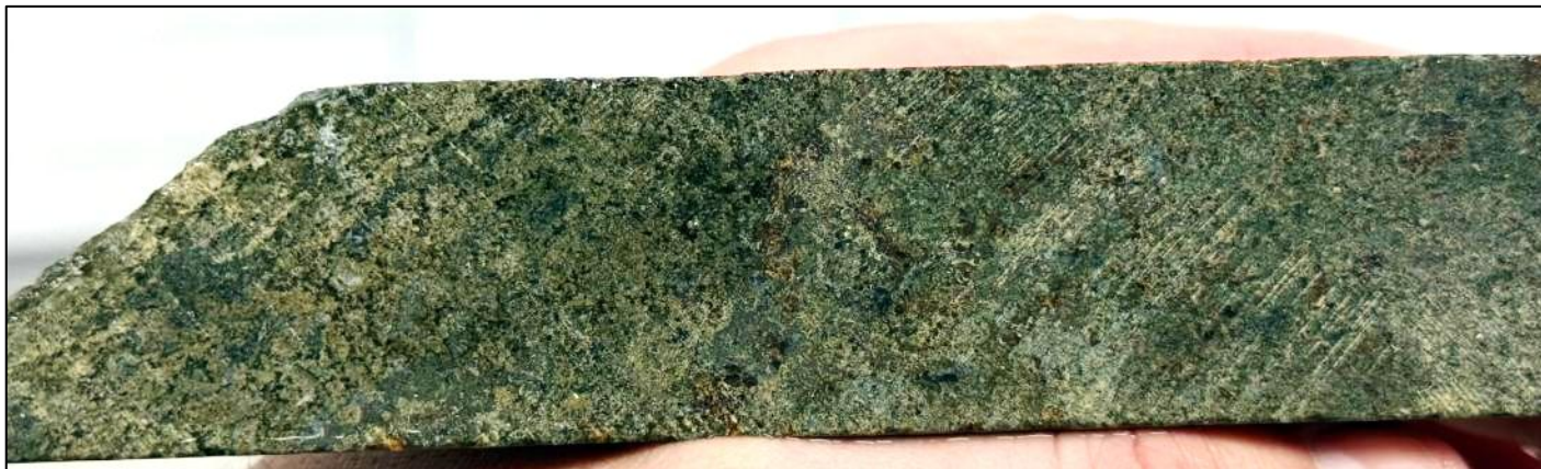
Figure 7. Core photograph from 517.5m to 519.5m in ZRSD25225 showing green garnet skarn with disseminated pyrite-chalcopyrite-sphalerite-arsenopyrite – 5.8g/t Au.
