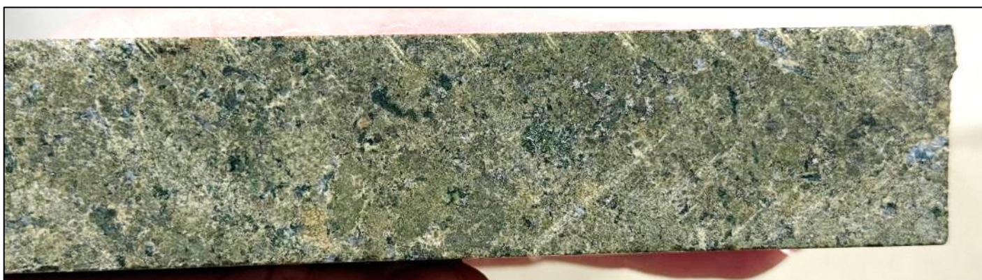
Figure 5. Core photograph from 580.0m to 582.0m in ZRSD25216B, showing green garnet skarn with disseminated pyrite-pyrrhotite-arsenopyrite – 6.7g/t Au.
