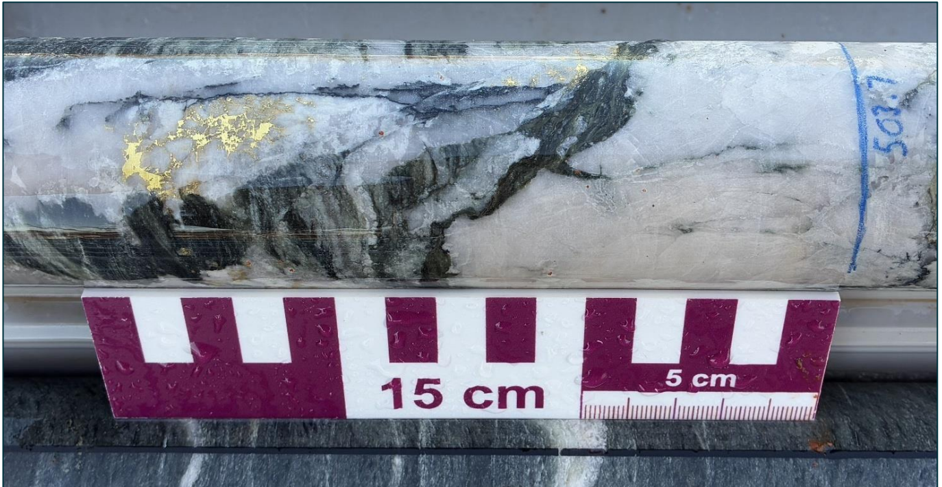
Figure 4: Coarse gold from 503.52 to 503.66m down-hole in 25MBRCD002A
