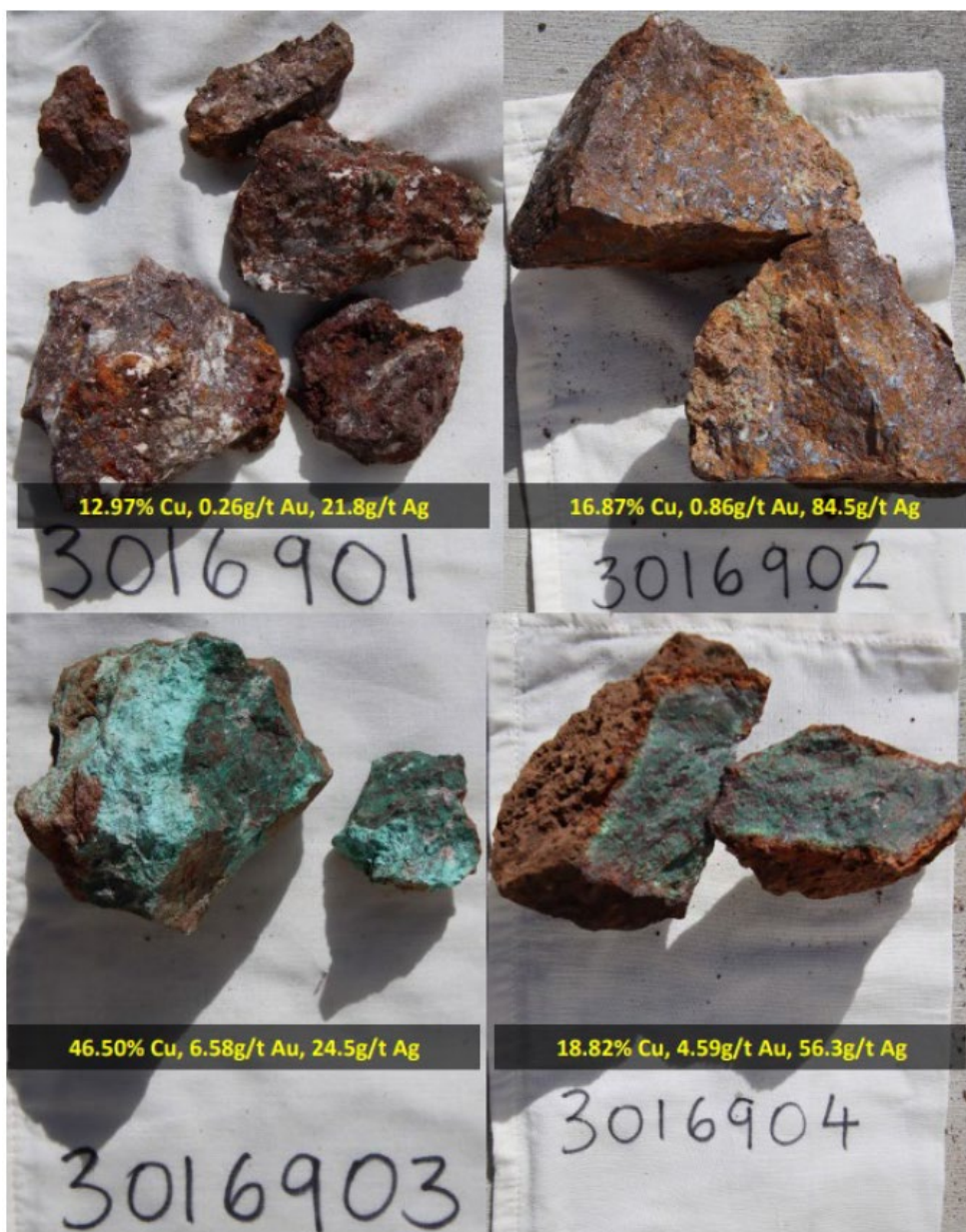
Figure 13. Mullock and rock chip samples collected from the Halls Reward Prospect. Sample 3016901 – copper oxide bearing ferruginous quartz, native copper and malachite; Sample 3016902 – copper oxide bearing ferruginous quartz, native copper, cuprite and malachite; Sample 3016903 – copper oxides chrysocolla and malachite; and sample 3016904 – copper oxide bearing ferruginous siliceous gossan, malachite needles, cuprite, spongy silica. 14
