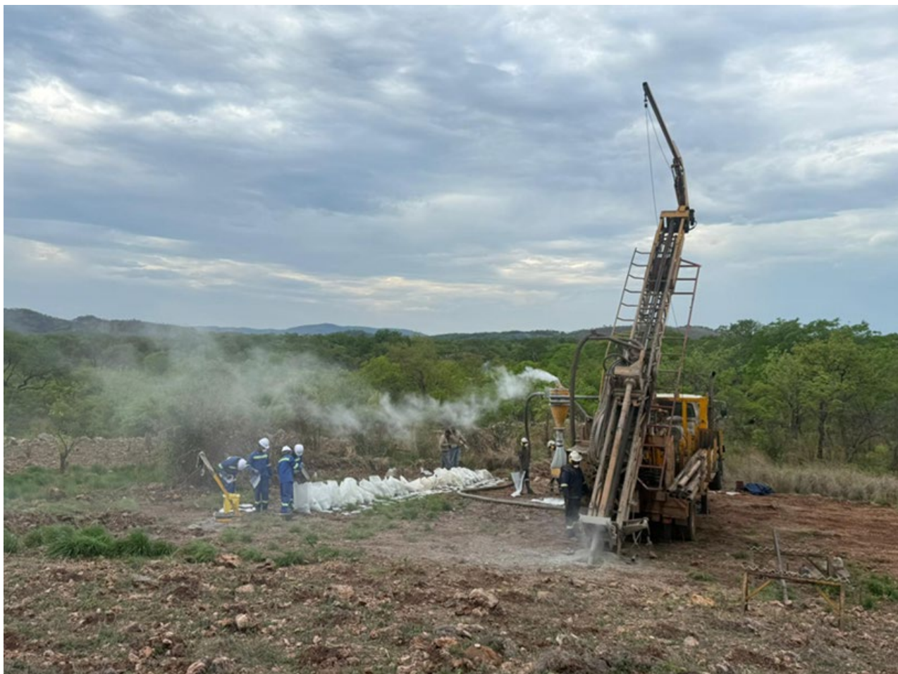
Figure 1: RC drilling at Aucu at the Chewbacca prospect, targeting quartz–sulphide–alteration structures within near-surface volcanic and intrusive units. Sample bags align in preparation for geological logging and assay submission.
