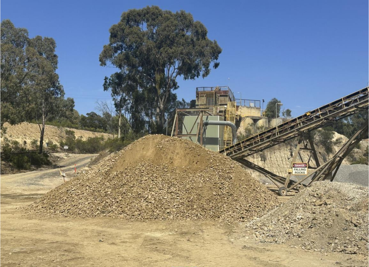
Figure 11. Union Hill Mullock material ready to be processed
