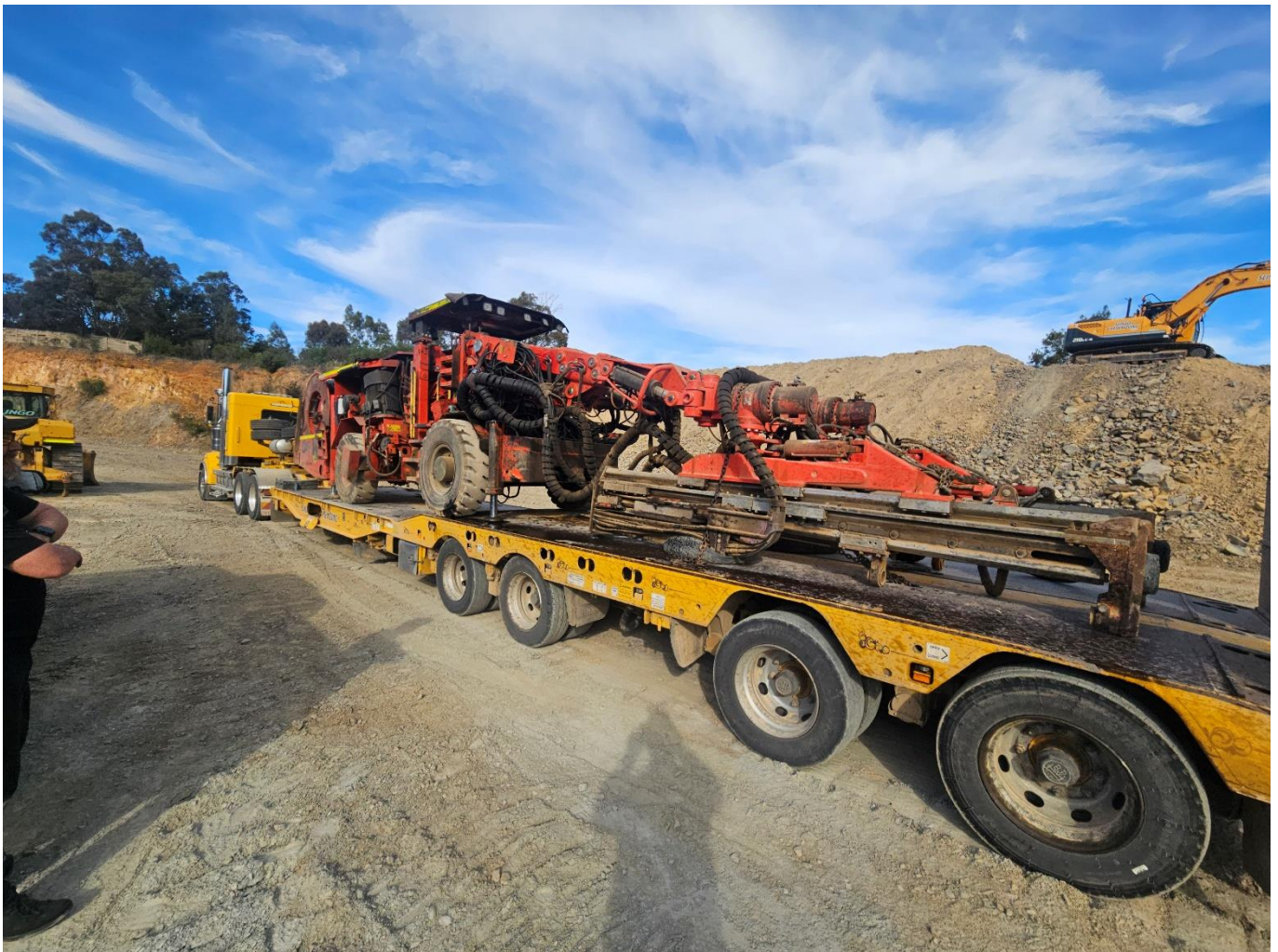
Figure 3. Twin Boom Jumbo delivered to Union Hill
