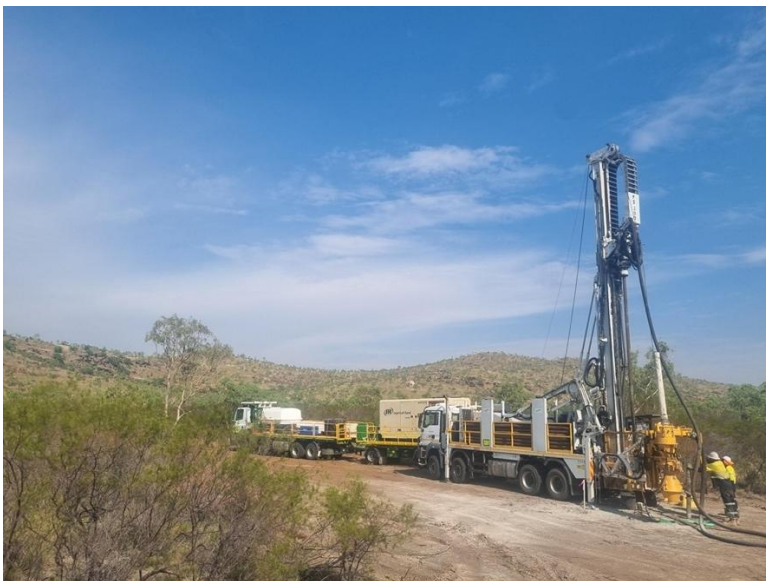
Figure 11: RC drill rig set up on Hole 24RCDH03
