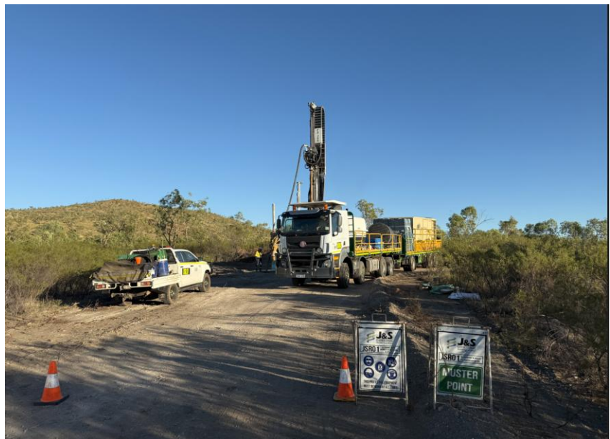
Figure 10: RC drill rig set up on Hole 24RCDH02
