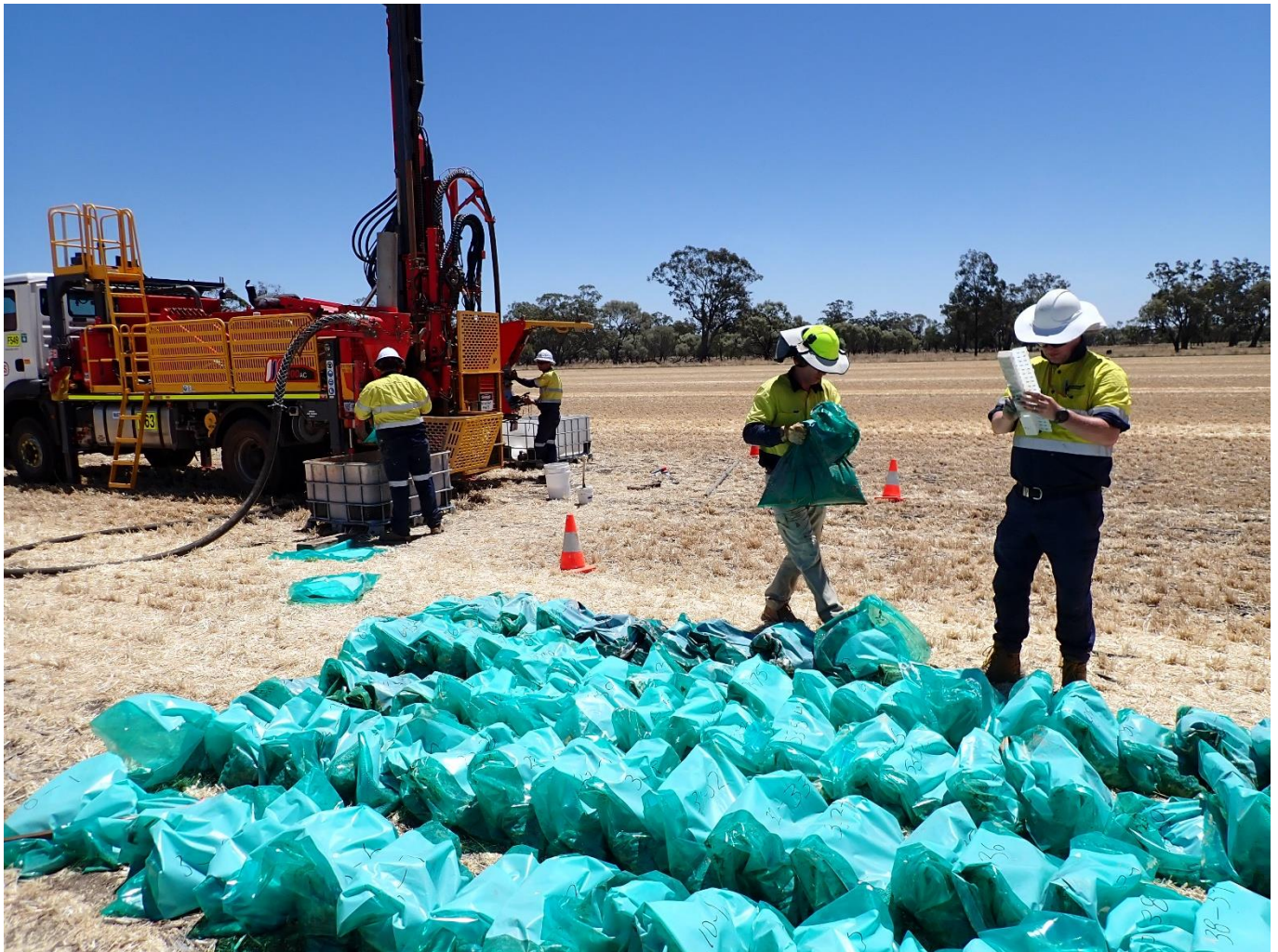
Figure 8: AC drilling at FJ Prospect with Magmatic staff
