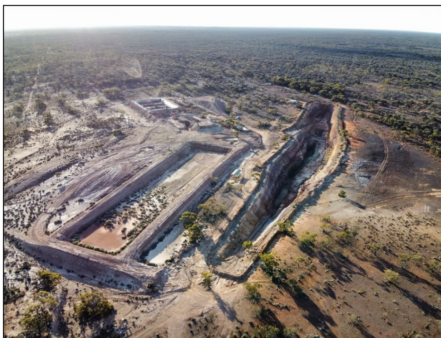
Figure 8: Drone photo of Zelica Project looking NNW showing pre-stripped open pit (approx. 300-400m long and 10-25m deep) and pre-constructed vat leach ponds (pic taken August 2025)
