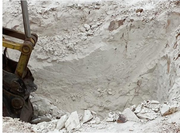
Figure 4: White Kaolin being excavated from the test pit
