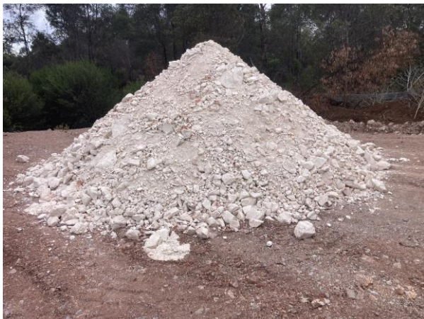
Figure 1: White Kaolin DSO excavated from the test pit
