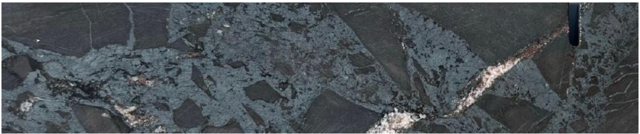
[Figure 8] Gulf Project: Hematite breccia from GTK2101 previously drilled on the Gulf project (refer Red Metal ASX release dated 27 January 2022).
