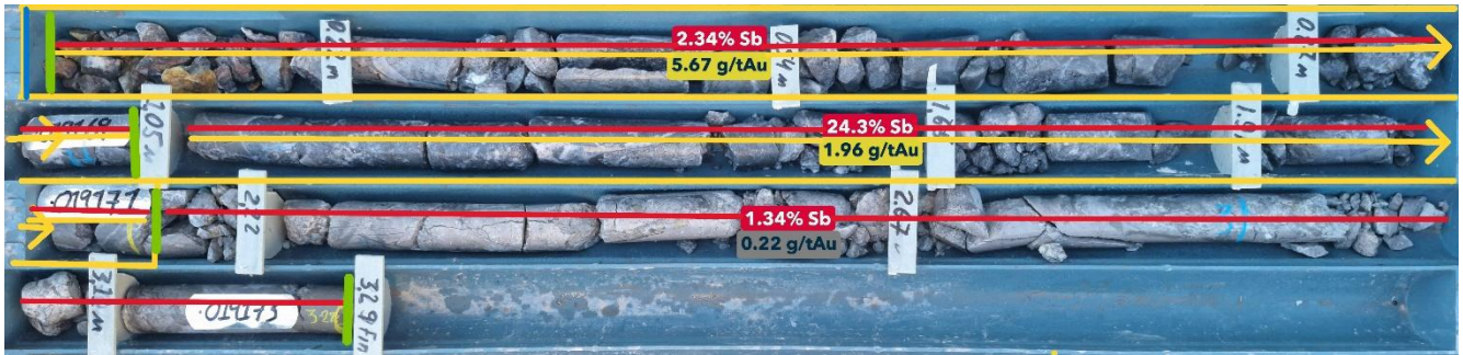
Figure 5 Photo of the core from drillhole UG25ZOP018 showing distribution of sample intervals and assay results.
