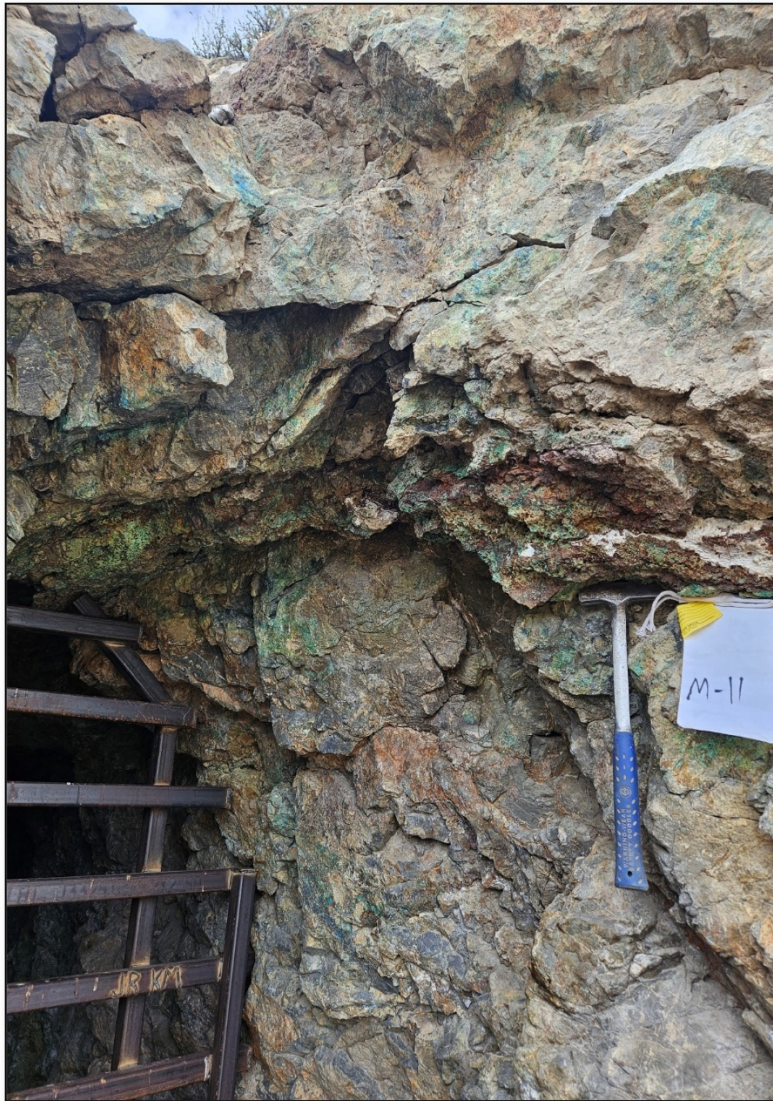
Figure 3: Tramway Adit: sample M-11 returned 24.0% Cu and 1.53% Sb, 434ppm Ag and >10,000ppm As from a 15cm wide central part of fault, within a broader 2m wide weakly faulted zone.
