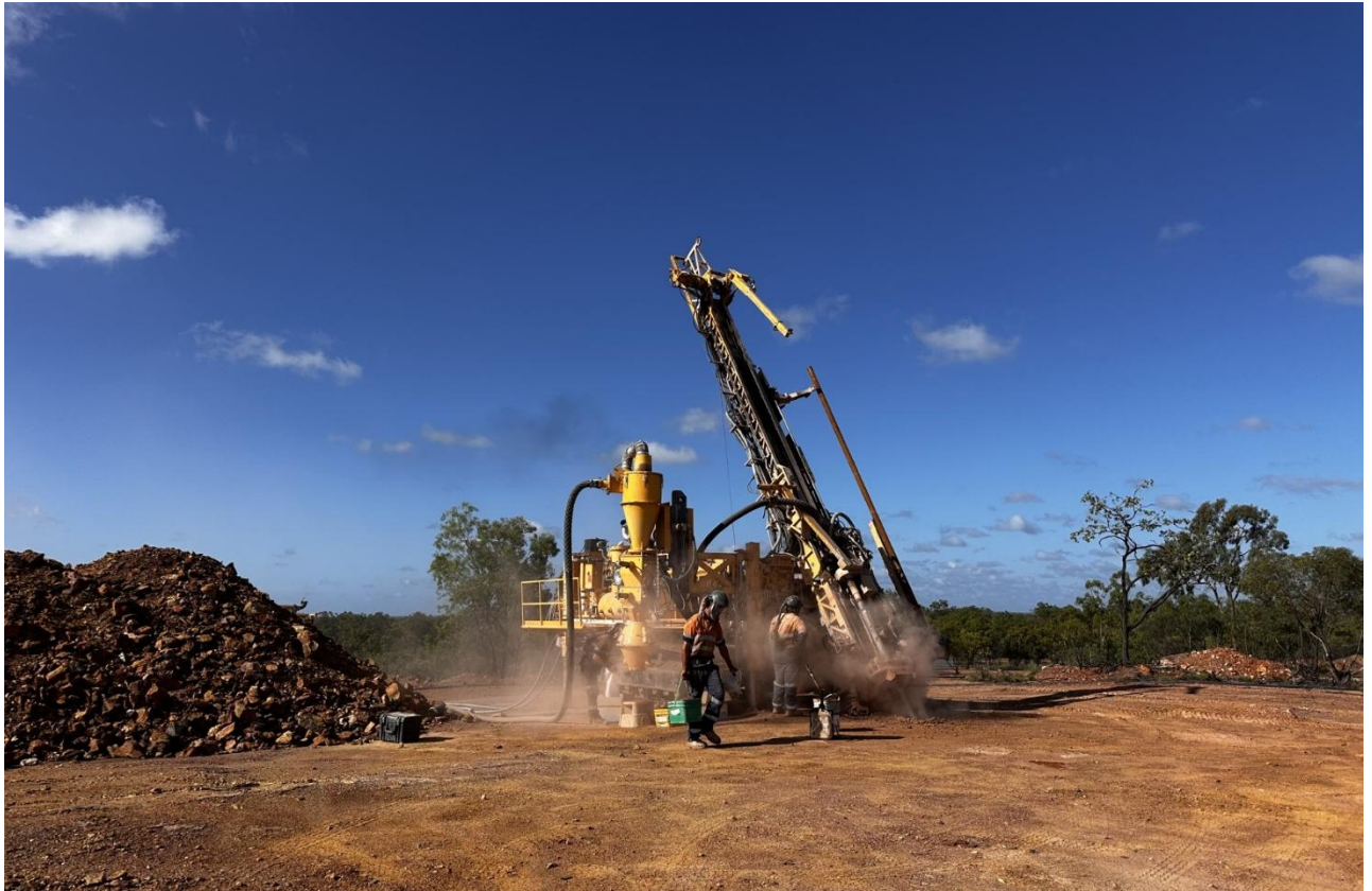
Figure 2: RC grade control rig drilling at Liontown.
