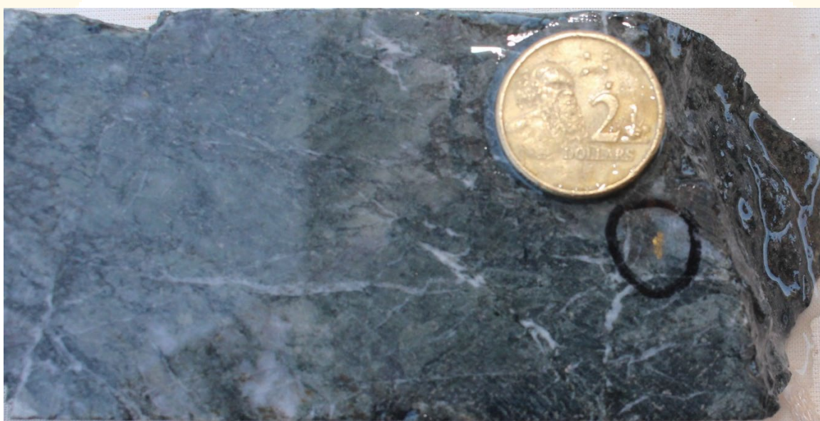
Figure 4: Visible gold within HYRCD25002 (235.25-235.45m) – sample interval with received grade of 26.9g/t Au – part of the intercept of 9m @ 4.3g/t Au from 233m including 2m @ 17.8g/t Au from 234m reported above
