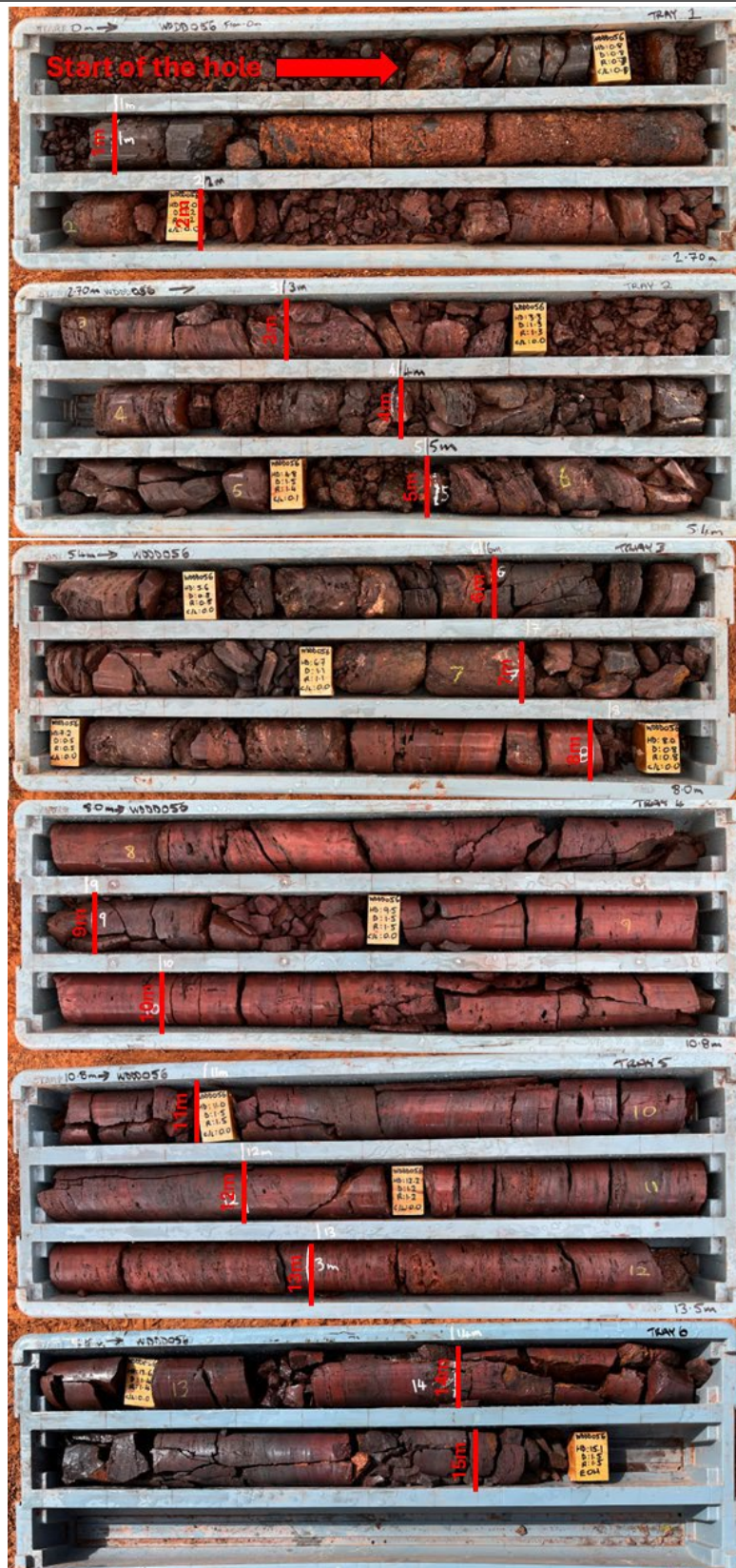
Figure 10: Drill hole WDD056 twinning hole WDRC056 that intersected 13m @ 59.3% Fe & 0.7% Mn from 1m including 7m @ 62.0% Fe & 0.7% Mn from 7m. Assays quoted from the equivalent interval from WDRC056 to the twin diamond hole will vary due to geological variation and recovered core. High grade iron mineralisation can be observed from 8 to 14m depth. Downhole metre marks are drawn on the core and tray ribs.
