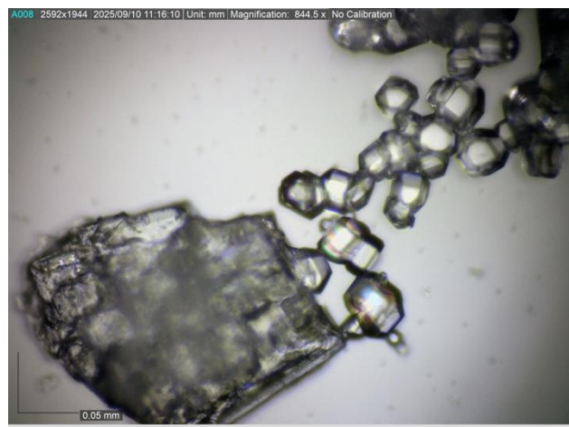
Figure 1. Crystals of high-purity Sulphate of Potash ( K_2SO_4 ) produced by direct membrane crystallisation, offering lower Capex and Opex compared to conventional SOP crystallisers.
