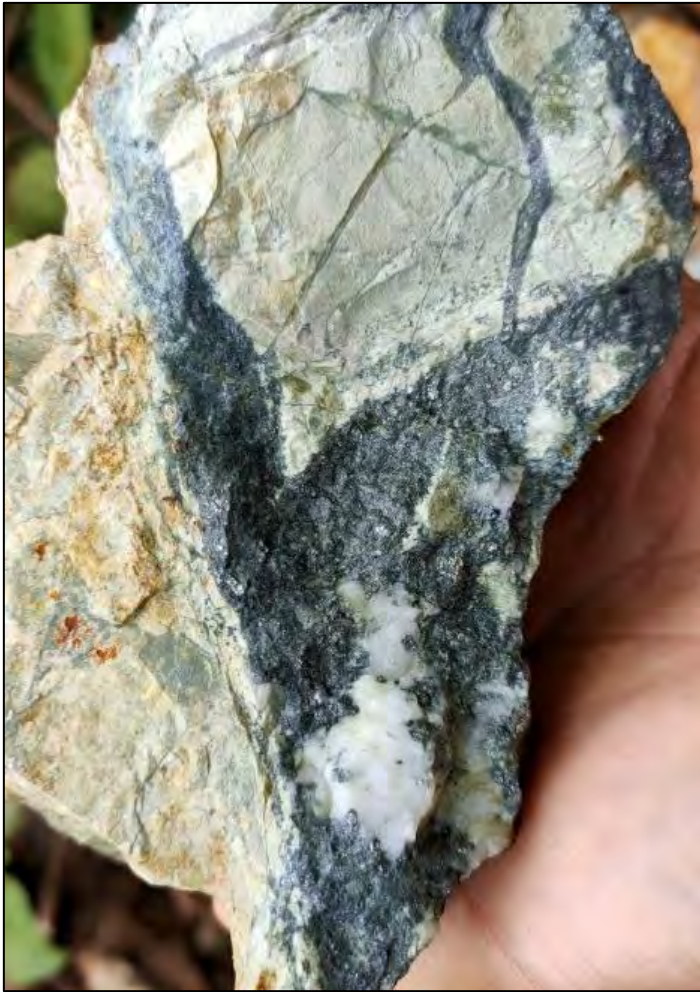
Photograph 3. Quartz-arsenopyrite breccia from the Ngot NE Prospect. A grab rock chip sample taken from this vein returned 2.2 g/t gold (sample number 103090). Details on the results of Unity Metals sampling of this vein are provided in the Independent Geologist's Report. All of the rock chip sample results from the Ngot Gold Project are provided in Appendix A of that report.
