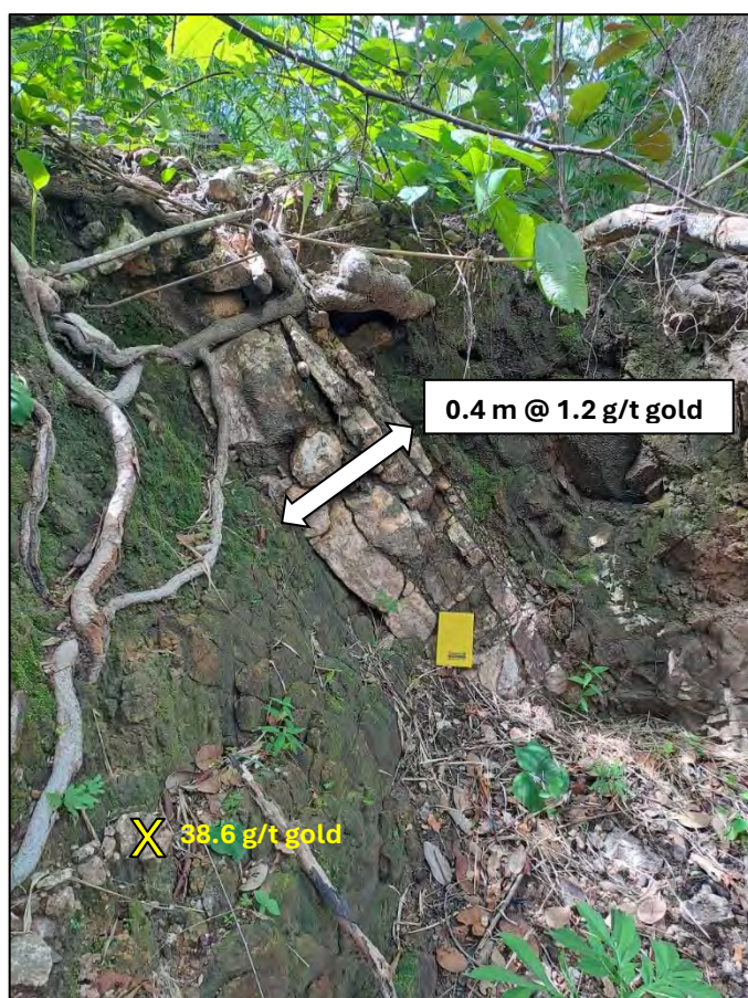
Photograph 1. New artisanal workings at the Ngot Central Prospect on shallow dipping, stacked, banded quartz – arsenopyrite veins hosted in weathered diorite (2 m below surface). A vertical composite channel rock chip sample result of 0.7 m @ 6.5 g/t gold was obtained (sample numbers 103304-103306). Details on the results of Unity Metals' sampling of these veins are provided in the Independent Geologist's Report. All of the rock chip sample results from the Ngot Gold Project are provided in Appendix A of that report.
