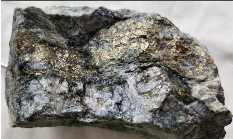
Photograph 5. Gold-bearing quartz-pyrite-pyrrhotite-chalcopyrite vein that extends SSW from the Mesam Gold Mine into the Ngot Gold Project. A grab rock chip sample taken from this vein returned 6.2 g/t gold, 202 g/t silver, 1.3% copper and 680 g/t bismuth (sample number N2306010). Details on the results of Unity Metals' sampling of this vein (which is exposed in artisanal workings and lies 200 m outside of Unity Metals' Project area) are provided in the Independent Geologist's Report. All of the rock chip sample results from the Ngot Gold Project are provided in Appendix A of that report.
