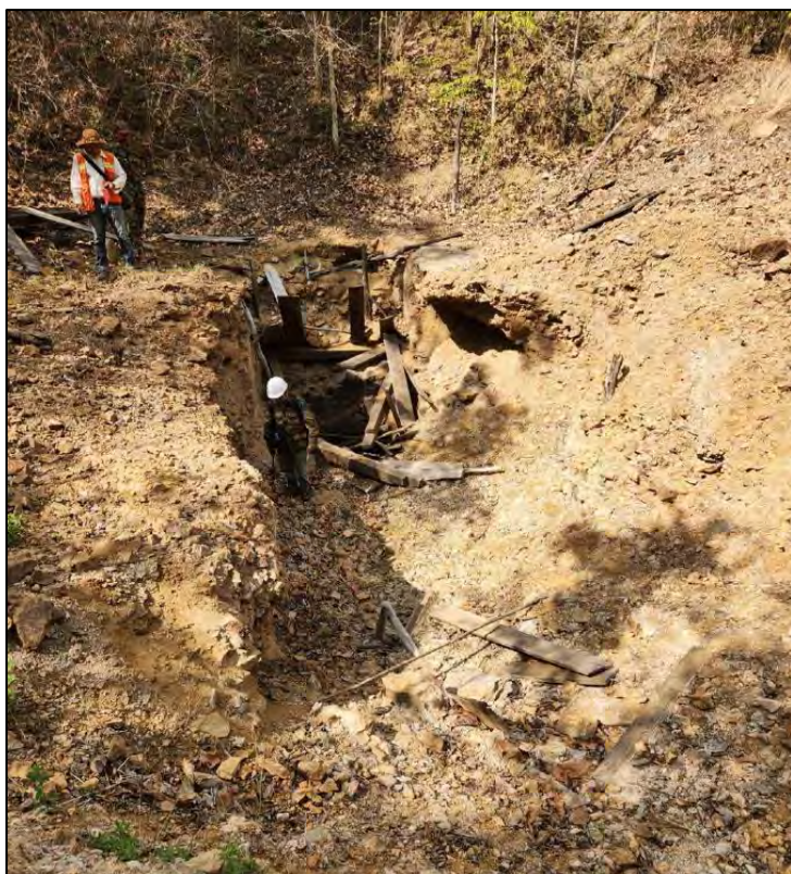
Photograph 25: Small Creek Prospect. Main, 2 m x 2 m, wooden-lined shaft in the historical workings. Source: Author.
