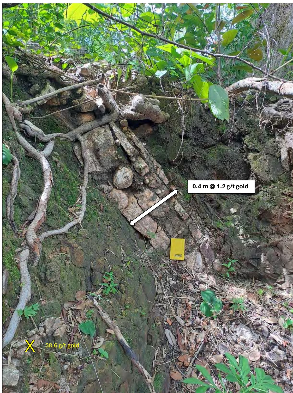
Photograph 4: Historical artisanal workings inspected by the Author at the Ngot Central Prospect on gold-bearing, banded, quartz-arsenopyrite veins hosted in weathered diorite. A channel rock chip sample (ID 103341) taken from a 40 cm wide stacked vein at location 689512 m East, 1391773 m North returned an assay result of 1.2 g/t gold. A grab rock chip sample (ID 103344) taken from a stock work vein at location 689524 m East, 1391774 m North returned assay results of 38.6 g/t gold and 21.6 g/t silver (refer to Appendix A for all rock chip sample assay results). Source: Unity Metals.
