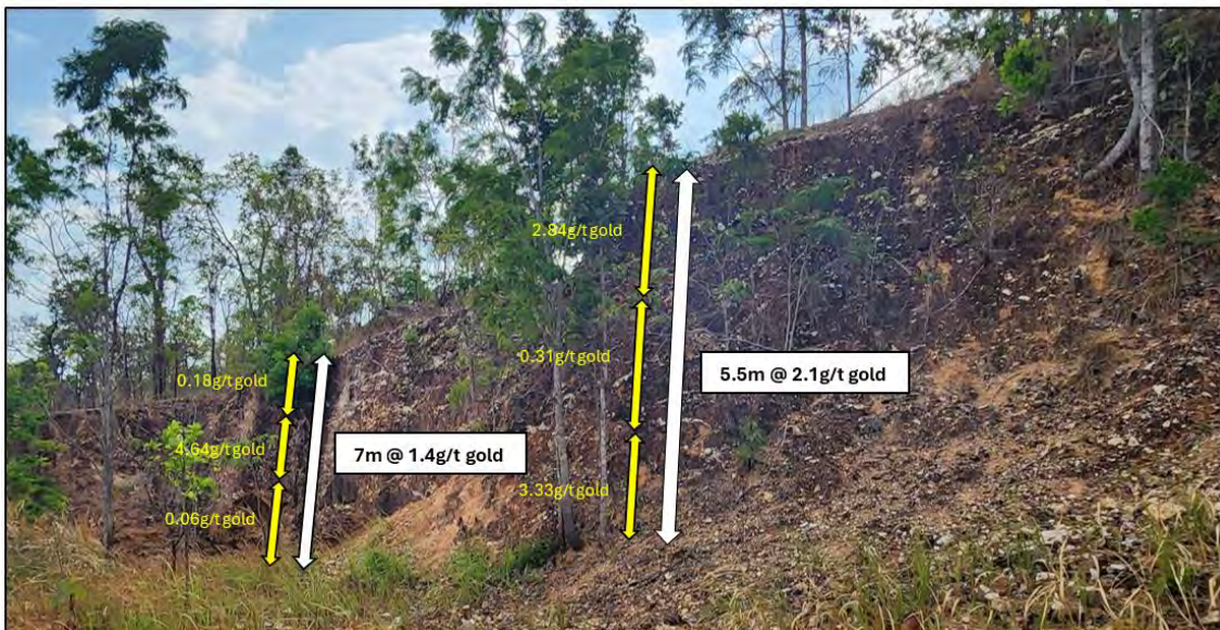
Photograph 7. Historical gold workings at the Camp Prospect on intense stockwork quartz-arsenopyrite vein mineralisation hosted in granodiorite (looking SW). Given the shallow dip of the mineralisation, Unity Metals collected vertical channel rock chip samples from exposed pit walls. Composite channel rock chip sample results include 5.5 m @ 2.1 g/t gold (sample numbers O2303021 – O2303023) and 7 m @ 1.4 g/t gold (sample numbers O2303018 – O2303020). Details on the results of Unity Metals' sampling of this mineralisation are provided in the Independent Geologist's Report. All of the rock chip sample results from the O'Phlay Gold Project are provided in Appendix B of that report.
