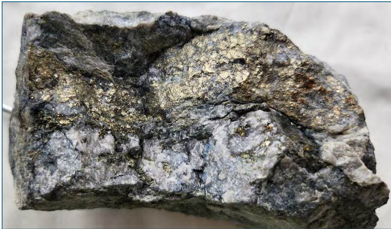
Photograph 16: Gold-bearing quartz-pyrite-pyrrhotite-chalcopryite vein that extends south-southwest from the Mesam Gold Mine towards the Ngot Gold Project. A rock chip sample (ID N2306010) taken from this vein in artisanal mine workings at location 703318 m East, 1393559 m North (200 m outside the Ngot Gold Project) returned assay results of 6.2 g/t gold, 202 g/t silver, 1.3% copper and 680 g/t bismuth (refer to Appendix A for all rock chip sample assay results). Source: Unity Metals.
