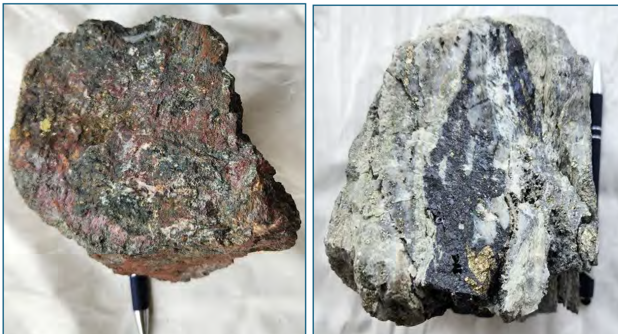
Photograph 7: (Left) Ngot Central Prospect. Float sample of diorite with chalcedonic quartz veins and quartz vein breccia with disseminated chalcopryrite and possibly cuprite. A rock chip sample (ID N2303048) taken from this mineralised diorite at location 689112 m East, 1391672 m North returned assay results of 44 g/t gold, 119 g/t silver and 1.1% copper (refer to Appendix A for all rock chip sample assay results). Source: Unity Metals.
