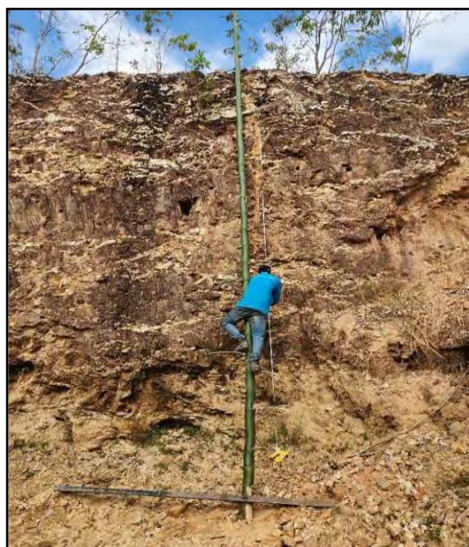
Photograph 19: (Left) Camp Prospect. Channel rock chip sampling of the intense stockwork mineralisation which is exposed in pit walls associated with the historical mine workings south of the abandoned processing plant at the Camp Prospect. Source: Unity Metals.
