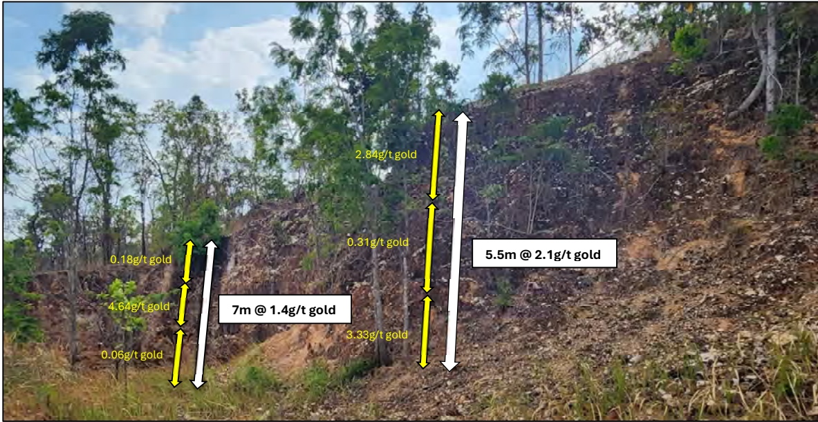
Photograph 18: Camp Prospect. Historical gold workings on intense stockwork quartz-arsenopyrite vein mineralisation hosted in granodiorite (looking SW). Given the shallow dip of the mineralisation, Unity Cambodia collected several vertical channel samples from exposed pit walls. The composite channel rock chip result of 5.5 m @ 2.1 g/t gold displayed in the photograph is comprised of the following individual channel rock chip assay results all located at 762782 m East, 1416144 m North: sample (ID O2303021) with 2 m @ 2.84 g/t gold (upper); sample (ID O2303022) with 2 m @ 0.31 g/t gold (lower). The composite channel rock chip result of 7 m @ 1.4 g/t gold displayed in the photograph is comprised of the following individual channel rock chip assay results all located at 762775 m East, 1416138 m North: sample (ID O2303018) with 2 m @ 0.18 g/t gold (upper); sample (ID O2303019) with 2 m @ 4.64 g/t gold (middle); and sample (ID O2303020) with 3 m @ 0.06 g/t gold (lower) (refer to Figure 28 for channel rock chip sample locations and gold results and Appendix B for all rock chip sample assay results). Source: Unity Metals.
