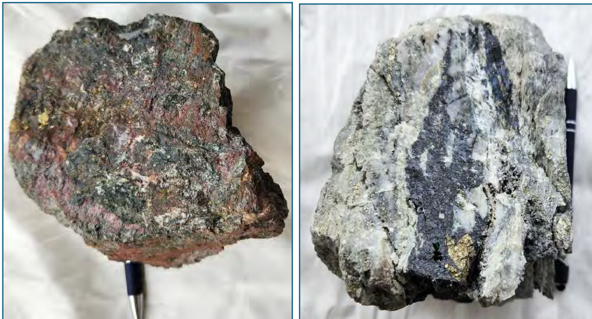
Photograph 7: (Left) Ngot Central Prospect. Float sample of diorite with chalcedonic quartz veins and quartz vein breccia with disseminated chalcopryite and possibly cuprite. A rock chip sample (ID N2303048) taken from this mineralised diorite at location 689112 m East, 1391672 m North returned assay results of 44 g/t gold, 119 g/t silver and 1.1% copper (refer to Appendix A for all rock chip sample assay results). Source: Unity Metals.
