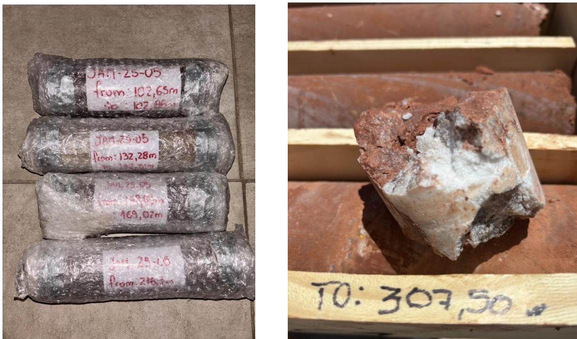
Figure 3. Four cores prepared for porosity testing and a sample of borate found at 307m depth indicative of lacustrine sedimentary deposits with lithium.
