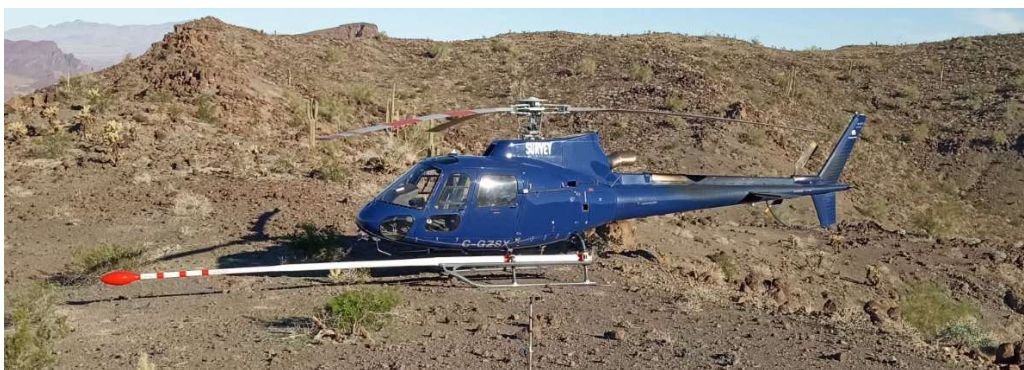
Figure 1 - Helicopter used for the ultra-high resolution airborne aeromagnetic and radiometric survey at the Parker Gold (Cu-Au) Project, shown at the base station magnetometer.
