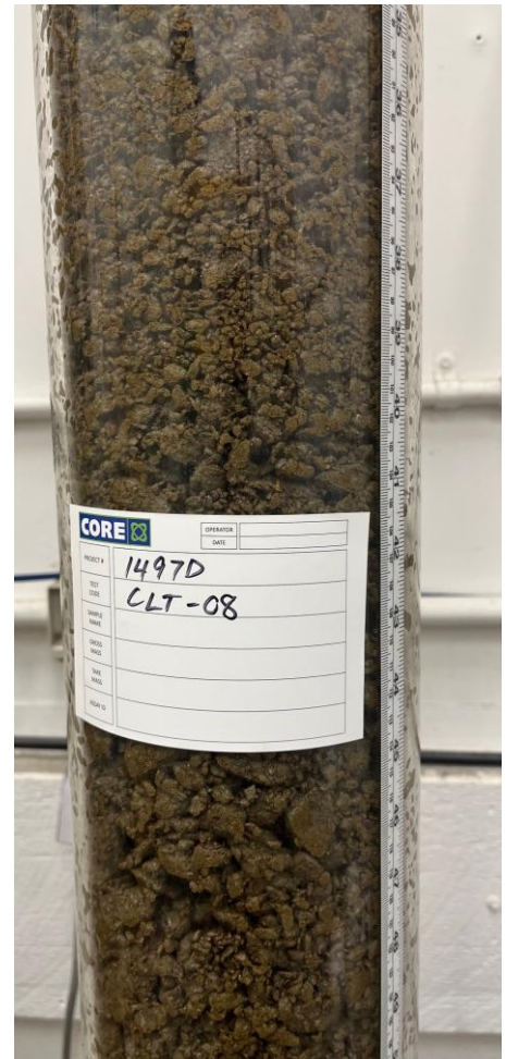
[Figure 1] Sybella Kary Zone Column Leach Tests in Progress: 2 metre by 100mm columns loaded with coarse -10mm and -20mm crushed mineralisation for a range of regolith types (left). Coarse crushed -20mm Transitional Granite – note the low-fines, very high porosity, and even acid saturation of the sample (right).
