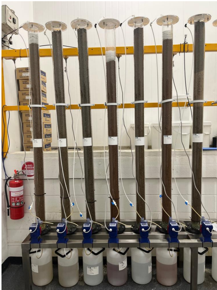
[Figure 1] Sybella Kary Zone Column Leach Tests in Progress: 2 metre by 100mm columns loaded with coarse -10mm and -20mm crushed mineralisation for a range of regolith types (left). Coarse crushed -20mm Transitional Granite – note the low-fines, very high porosity, and even acid saturation of the sample (right).
