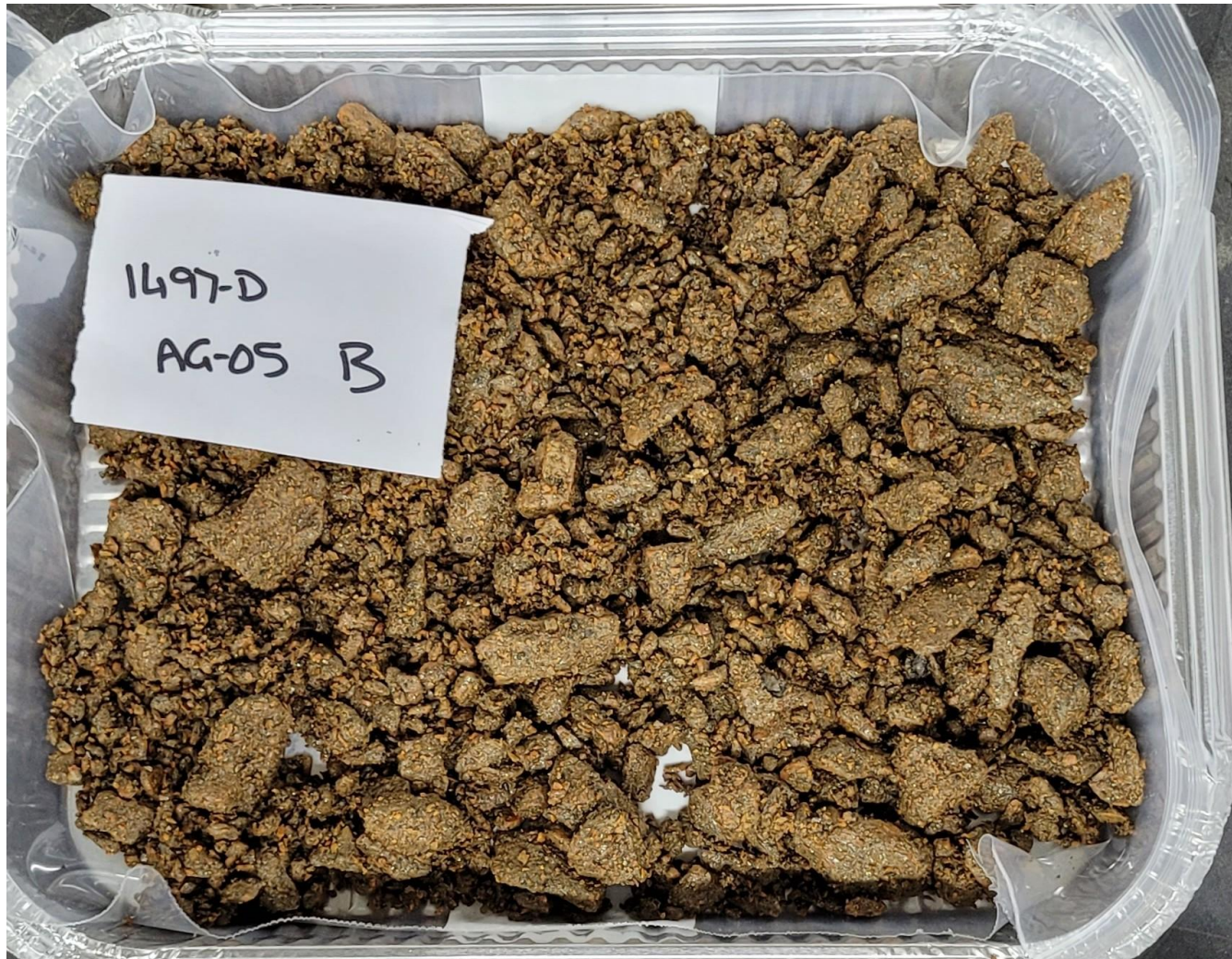
[Figure 2] Sybella Kary Zone Column Leach Tests: SC01 example of acid agglomerated -20mm crushed weathered granite. Note the fine chips from the crushing process bound (sticking) to the coarser fragments which helps to maintain a high permeability in the column.
