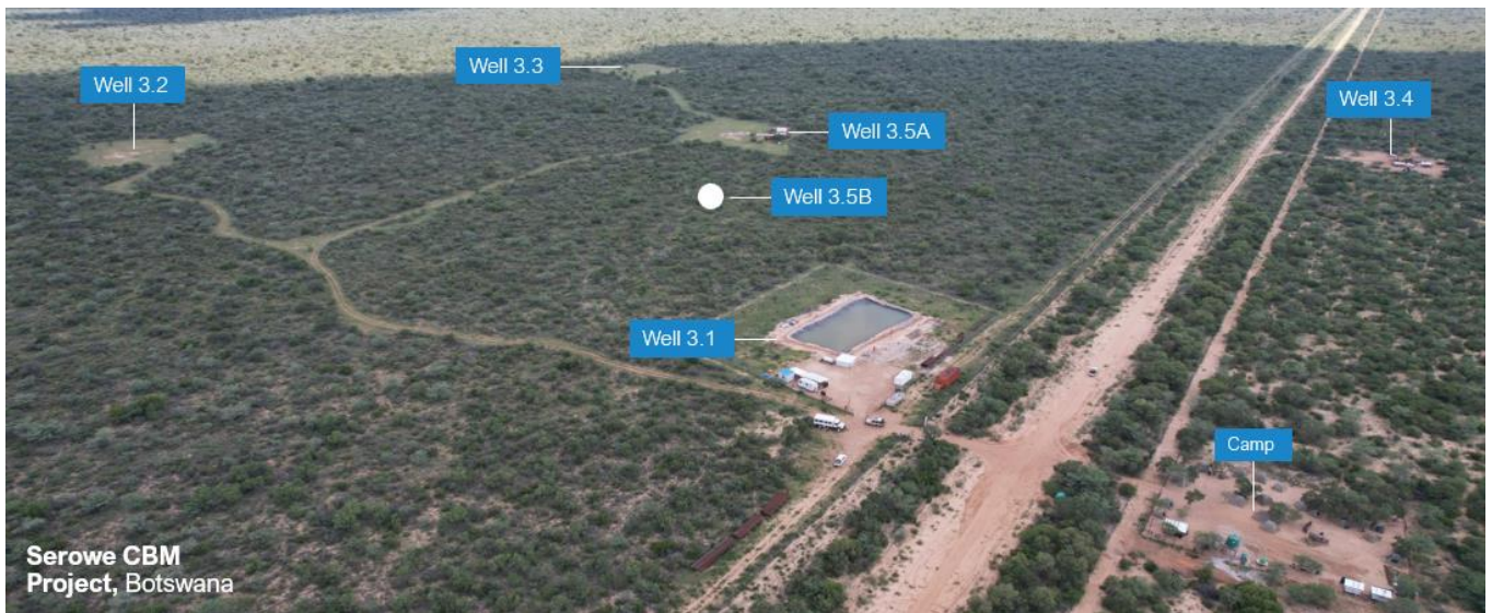
Figure 2. The first phase of Botala’s four-phase CBM to LNG plan is the delivery of Project Pitse, a proof-of-concept pilot made up of five producing wells (3.1 – 3.5B) and one central dewatering well (3.5A)
