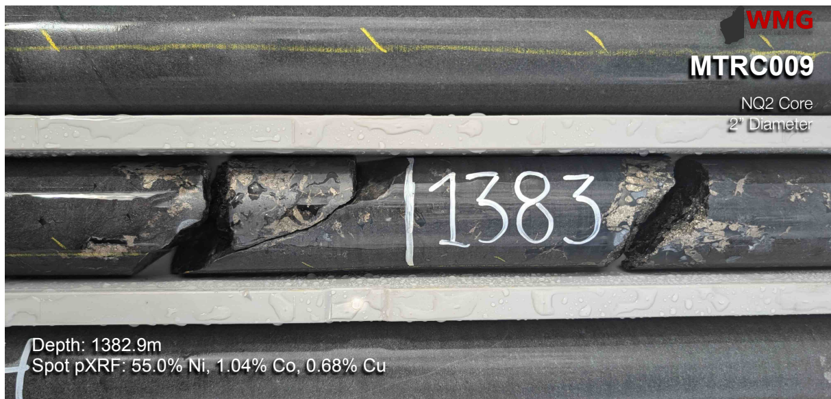
Figure 4: Photo showing examples of sulphide segregations in hole MTRC009 (EIS9)
