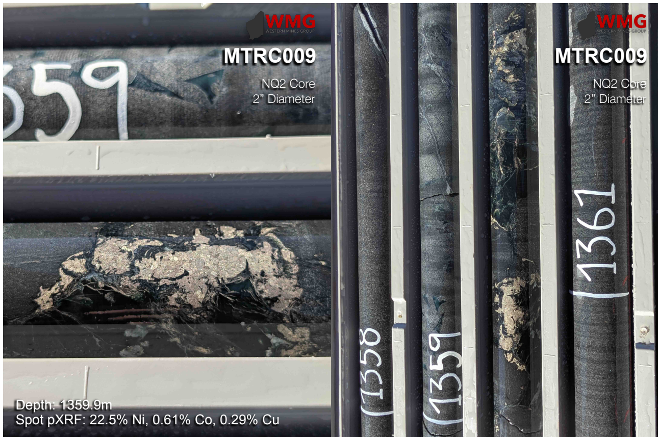
Figure 2: Photos showing examples of sulphide segregations in hole MTRC009 (EIS9) Note: core is NQ2 being 2 inches or 50mm diameter
