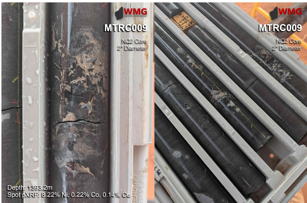
Figure 3: Photos showing examples of sulphide segregations in hole MTRC009 (EIS9) Note: core is NQ2 being 2 inches or 50mm diameter
