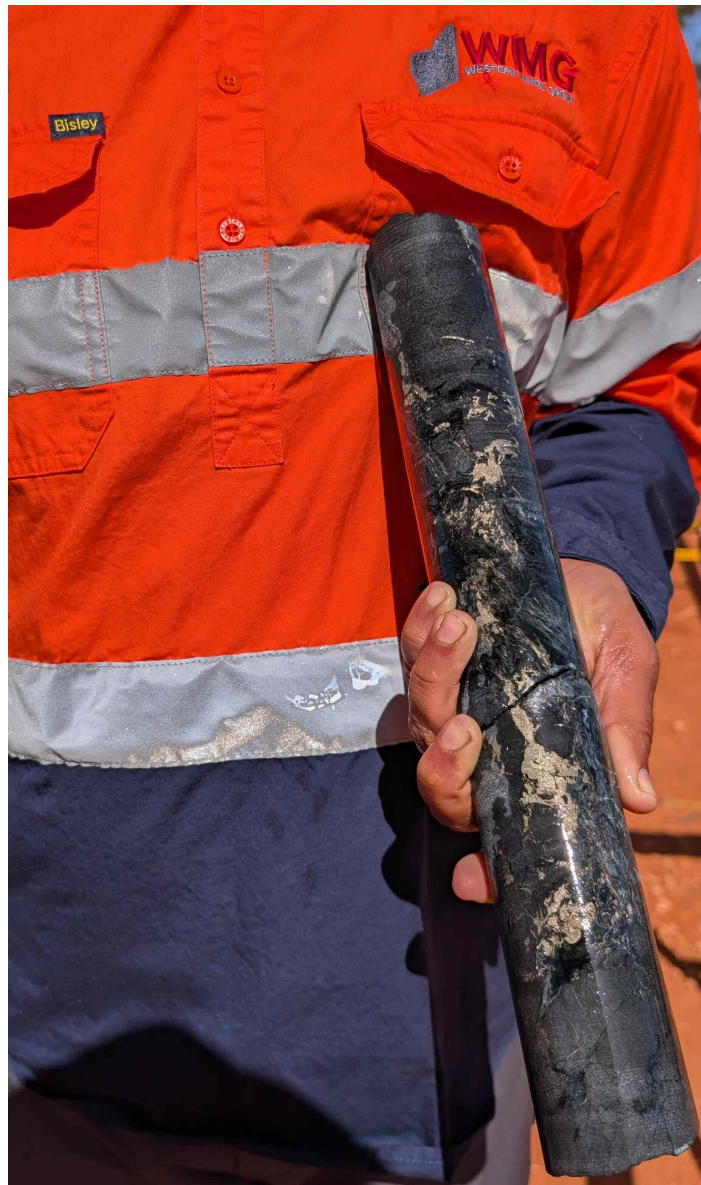
Figure 1: Photo showing example of sulphide segregations in hole MTRC009 (EIS9)
