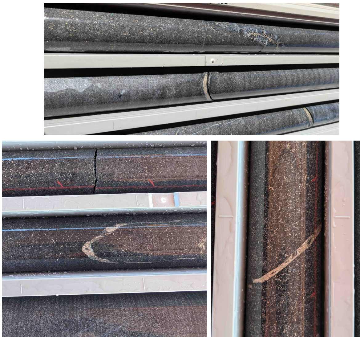
Figure 5: Photos showing examples of heavily disseminated sulphide in hole MTRC009 (EIS9)
