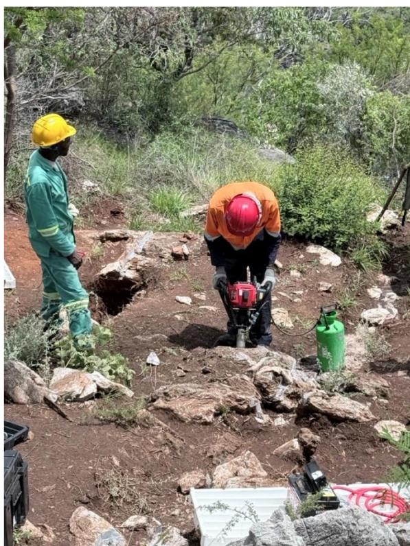
Images 2: Man-portable diamond rig testing Gossan 1 East. Image 3: Company personnel pulling rods with core enclosed
