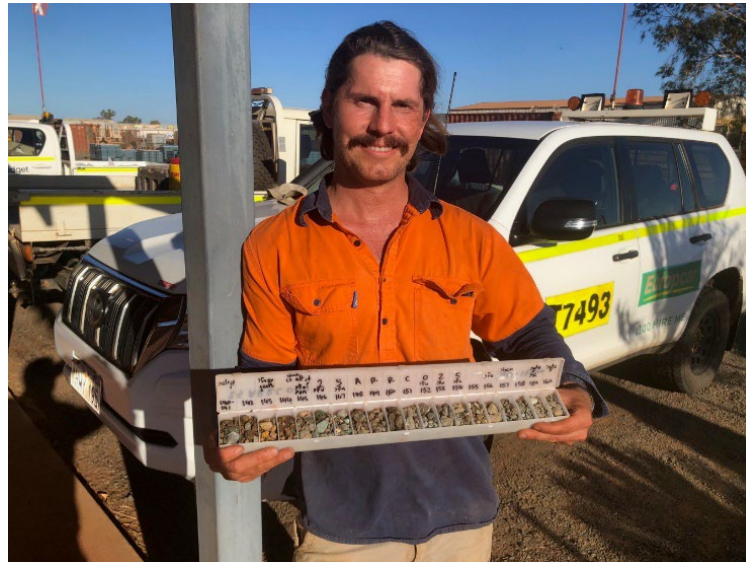
Figure 7: Project Geologist Tony Sheehan with drill chips from 25ARRC025 (140-160m) including veined, altered ultramafic sequence and sediments (Refer Table 3)
