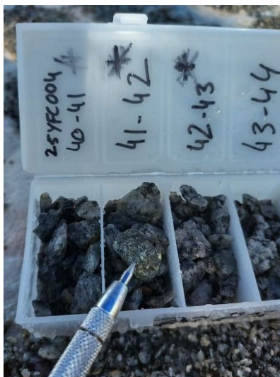
Photo 2: RC Drill Chips Showing Chalcopyrite from Drillhole 25YRC004 at 41-42m Depth
