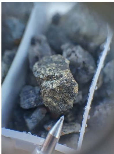
Photo 2: RC Drill Chips Showing Chalcopyrite from Drillhole 25YRC004 at 41-42m Depth
