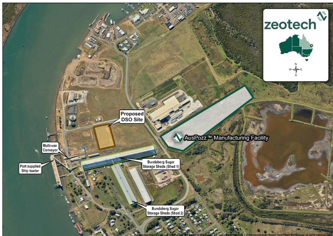
Figure 5: Proposed AusPozz™ Manufacturing Facility Area, Kaolin DSO storage site, and Multi-Use Conveyor (MUC) infrastructure located at the Port of Bundaberg, Queensland.
