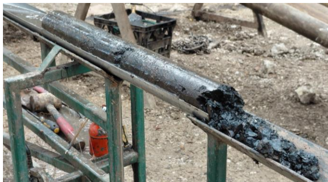
Figure 1: Drill-core from EMDD039, interval 10.70m – 11.70m, showing high-grade Mn mineralisation. Assay results summarised in Table 1 and detailed in Appendix 2.
