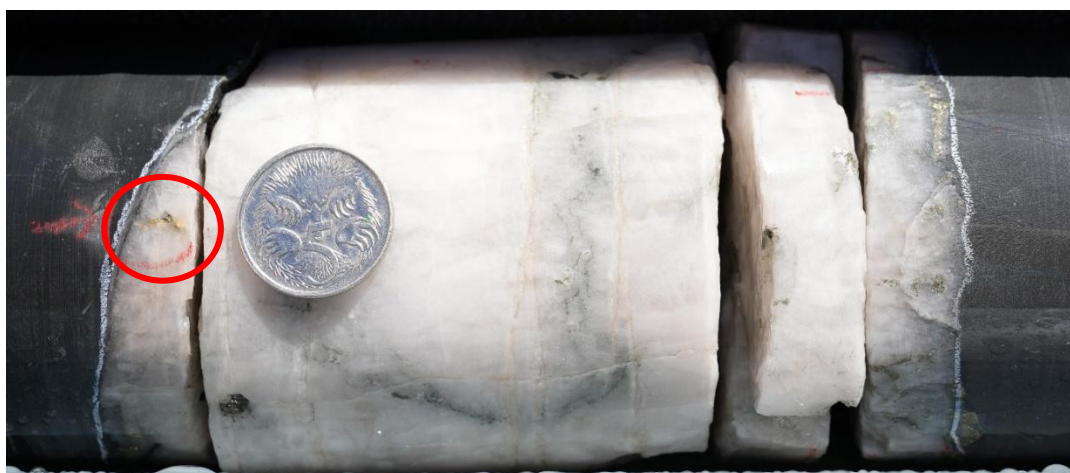
Figure 4 BMDD003 with visible gold (red circle) in an extensional quartz vein with pyrite near the vein margins at 605.6m
