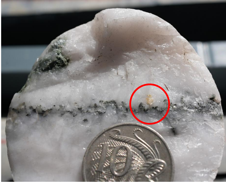
Figure 5 BMDD003 showing visible gold (red circle) in the stylolitic quartz carbonate vein at 607.6m
