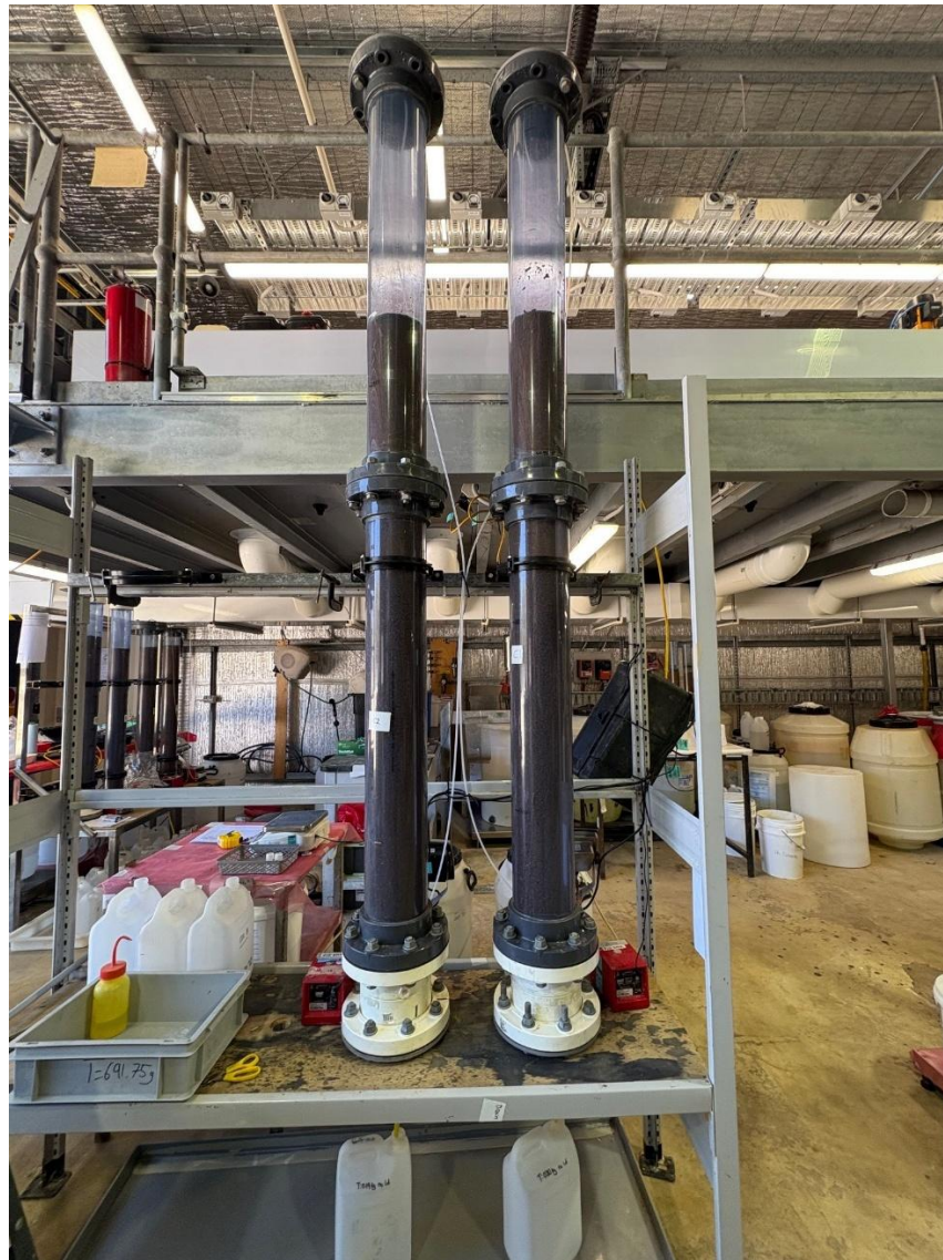
Figure 1: Column leach tests in progress at ANSTO on 26 kg samples from the ABx Deep Leads deposit
